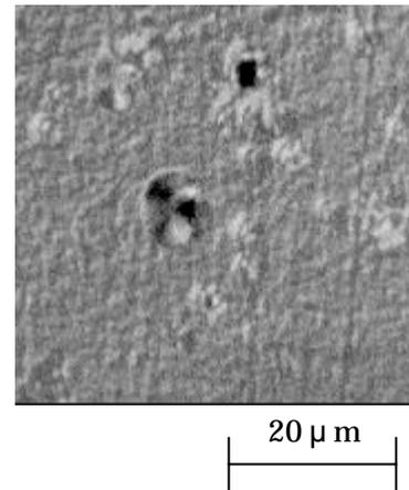
Fig.4. PMMA surface obtained by the conventional process taken by differentiation polarized light.
