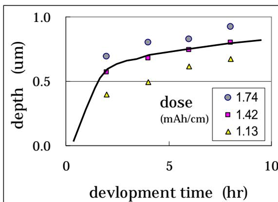
Fig.10 Etching depth dependence on the developing time for the 0.7 µ m thick PMMA
