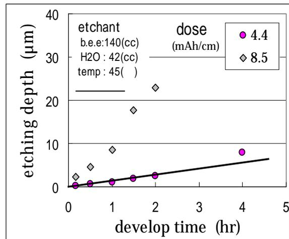
Fig.9. Etching depth dependence on the developing time for the commercial PMMA
