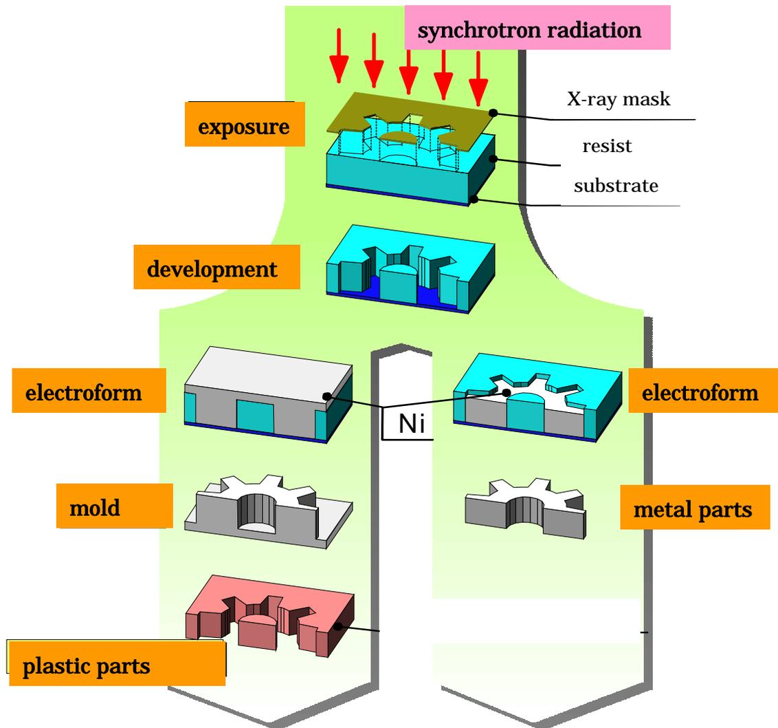
Fig.1. The conventional LIGA process
