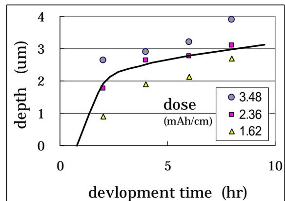
Fig.11. Etching depth dependence on the developing time for the 2.6 µ m thick PMMA
