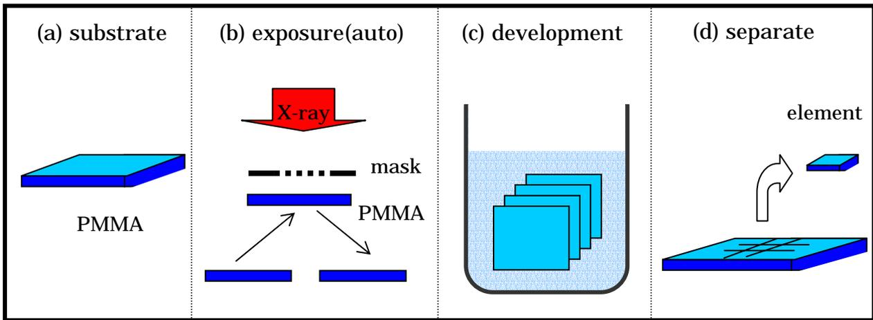
Fig.2 . Basic idea of the process
