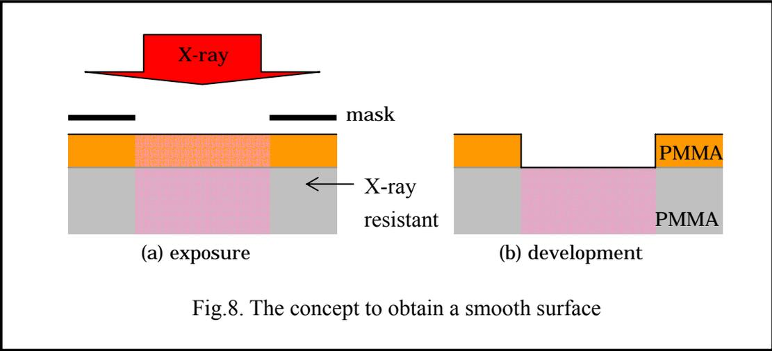
Fig.8. The concept to obtain a smooth surface
