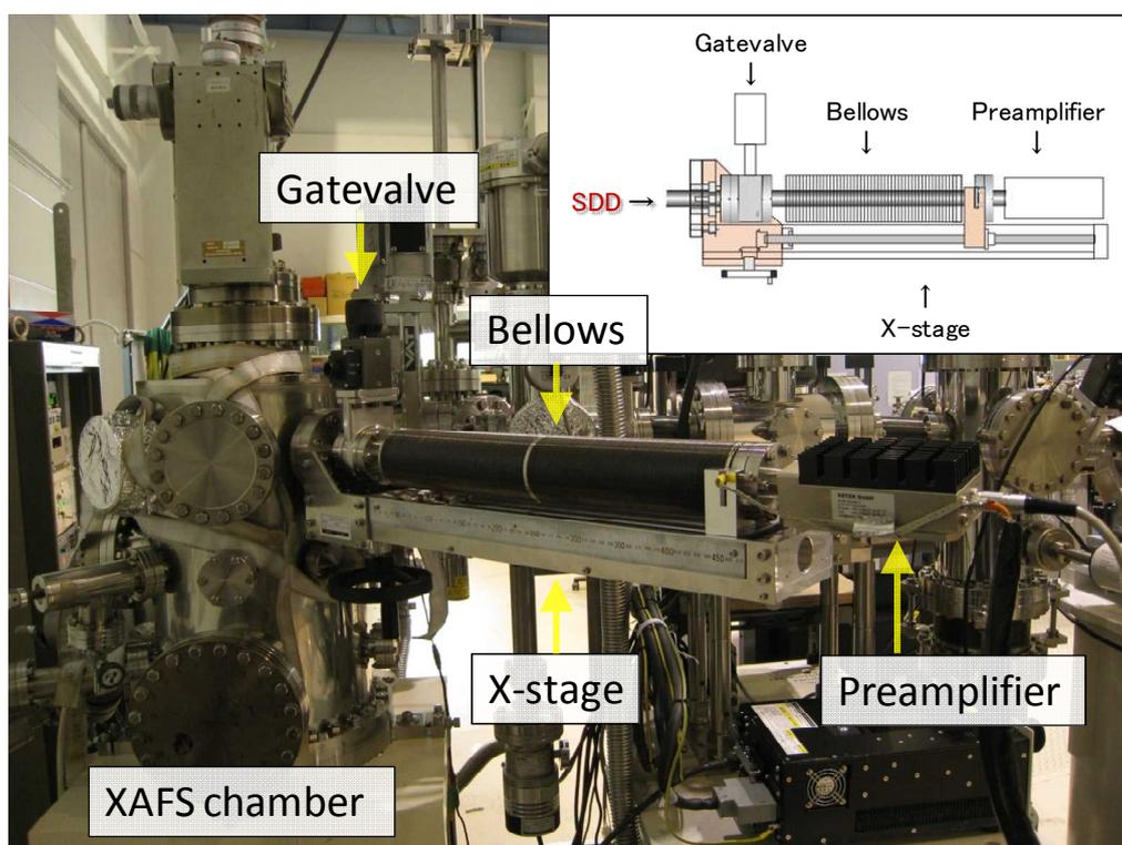
**Figure 1.** Outline of the large-area silicon drift detector.
