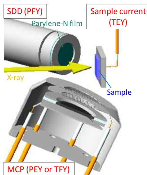
**Figure 3.** Setup for the simultaneous three-mode XAFS measurement.
