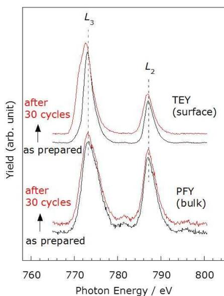
**Figure 5.** Co  $L_{2,3}$ -edge XAFS spectra of the  $\text{LiCoO}_2$  electrode soaked in the electrolyte solution and after 30 charge-discharge cycles.
