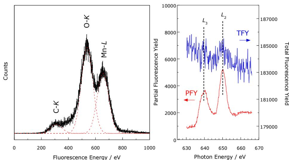
**Figure 4.** Fluorescence X-ray spectrum (left) and Mn  $L_{2,3}$ -edge XAFS spectra (right) of the  $\text{LiMn}_2\text{O}_4$  electrode.
