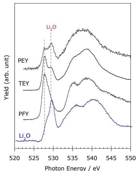
**Figure 6.** O  $K$ -edge XAFS spectra of the  $\text{LiCoO}_2$  electrode obtained by PEY, TEY and PFY methods.
