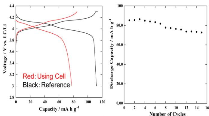
Figure 5. The battery capacity (A) and the cycle property (B) measured using the newly developed *in-situ* cell for the imaging XAFS measurements.
