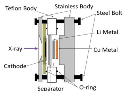
Figure 4. The schematic diagram of the electrochemical cell for *in-situ* XAFS measurement in soft X-ray region.
