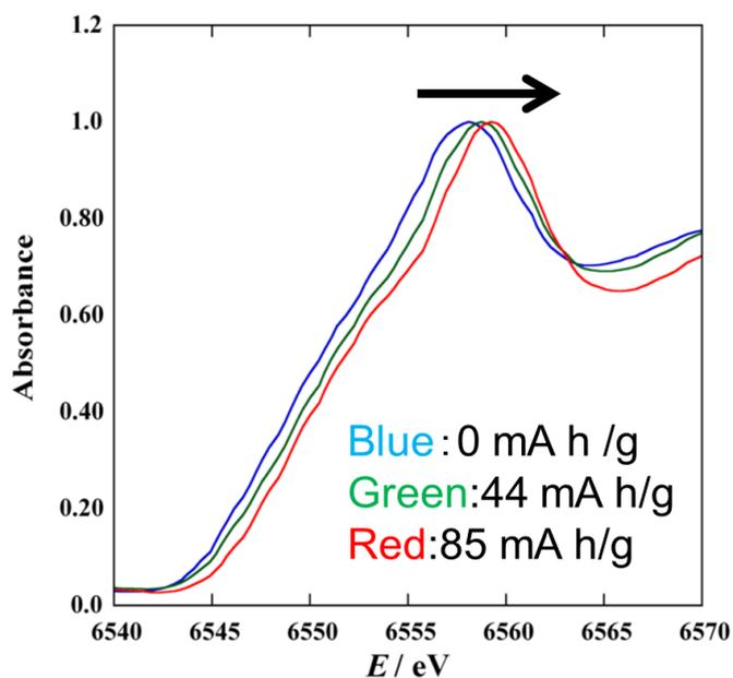
Figure 6. XANES spectral change during the charging reaction of the LMO cathode measured at the Mn K edge using the developed *in-situ* cell.
