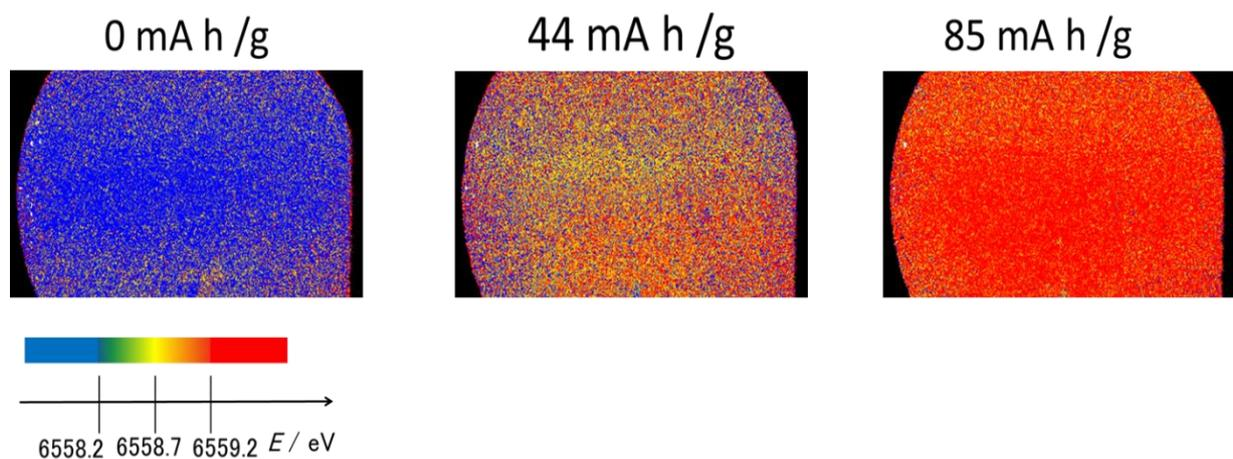
Figure 7. The chemical state map of the Mn species for the LMO cathode obtained by *in-situ* imaging XAFS measurement.
