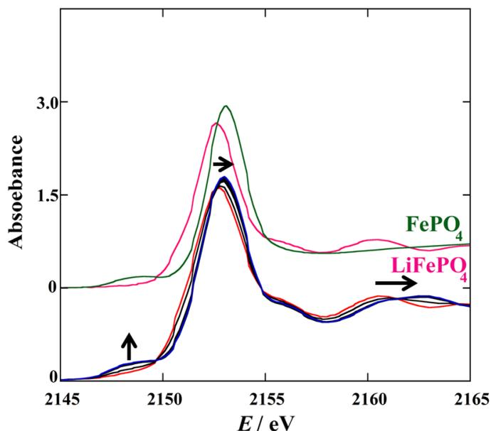
Figure 8. XANES spectral changed at the P K edge during the charging process of the LiFePO<sub>4</sub> cathode measured using the developed *in-situ* electrochemical cell for the soft X-ray region.
