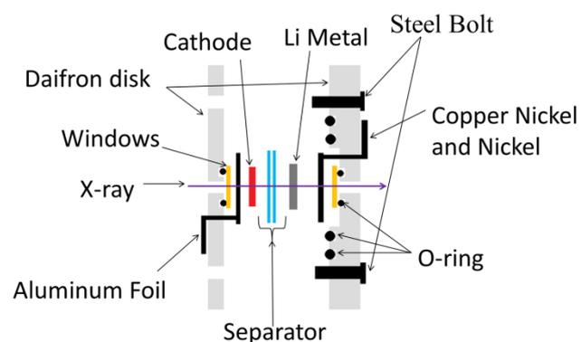
Figure 2. The schematic diagram of the electrochemical cell for imaging XAFS measurements.
