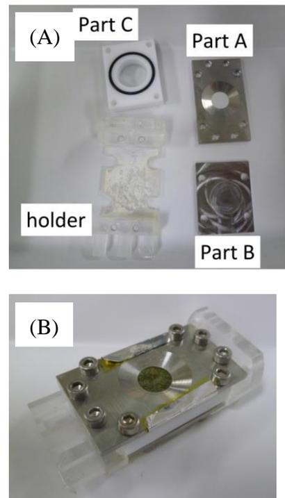
Figure 3. The picture of newly developed electrochemical cell for *in-situ* XAFS measurements in soft X-ray region.
