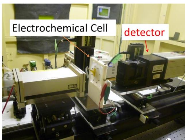
Figure 1. The picture of electrochemical cell for imaging XAFS measurements.
