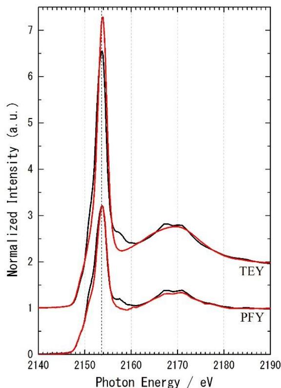
**Fig.2** P K-XANES spectra of SR irradiated (red) and non-irradiated (black) KTP crystal. Upper spectra are taken with the total electron yield mode (TEY) and lower are with the partial fluorescence yield mode (PFY).
