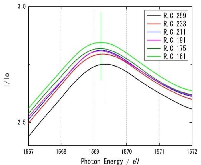
**Fig.1** Al K-edge XAFS spectra of aluminum foil.
