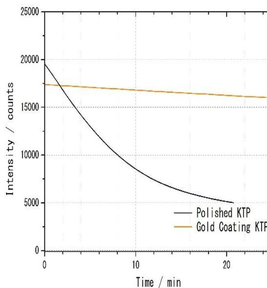
**Fig.3**  $I_0$  intensity of monochromatized beam from a bare KTP pair and a gold coated KTP pair as a function of the elapsed time. Ring current decay curve is also shown.
