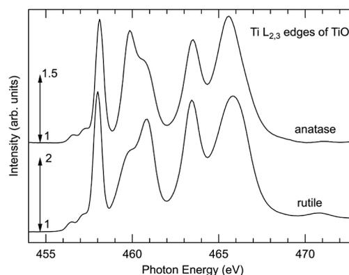
**Fig. 1.** Total electron yield spectra of anatase and rutile. The sample current is normalized using the current of Au mesh in front of the sample. The arrows and the numbers indicate the relative intensities at the ends of the arrows.
