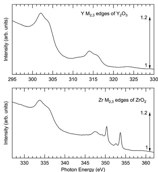
**Fig. 2.** Total electron yield spectra at the  $M_{2,3}$  edges of Y and Zr of  $\text{Y}_2\text{O}_3$  and  $\text{ZrO}_2$ . The arrows and the numbers indicate the relative intensities at the ends of the arrows. In the lower panel, the structures between 350 and 360 eV are presumably due to Ca contamination.
