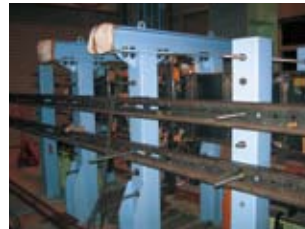
■ Experiment on the strength of a steel girder (Heavily deformed shape indicates the ductility of steel)
