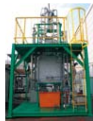
■ A pilot apparatus of biofiltration system for the preparation of its practical use. Unique structures are equipped in gas-flow and filter material (patent has been approved)
