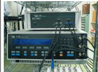
■ Impedance analyzer used in a dielectric relaxation spectroscopy method that enables dynamics measurements in wide time areas.
