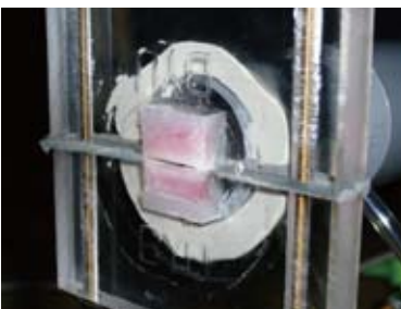
■ Physical model of vocal folds that can produce voice as human.
