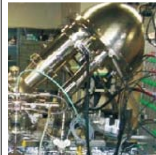
■ High-resolution photoemission apparatus, which precisely measures electrons escaping from a sample.
