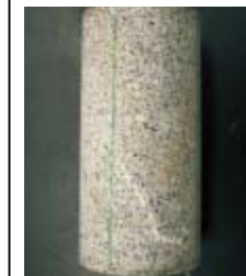
■ Granite sample on the way to fault formation. White part is a fault trace that will be a final rupture plane.
