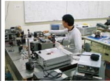
■ The spectrum width of a quantum cascade laser is measured to enable highly sensitive gas sensing.
