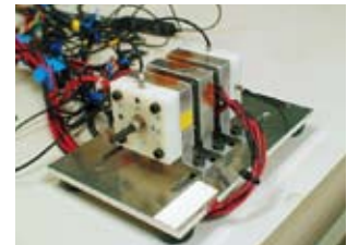
AC motor using small magnetic bearing
