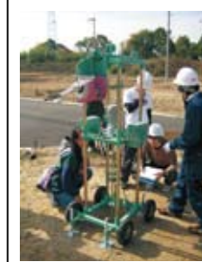
■ Carrying out a ground investigation in order to predict the subsidence of a building in a housing lot
