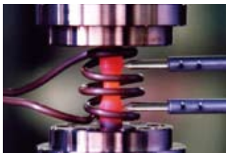
■ Multiaxial low cycle fatigue test of heat resistant steel using electro-hydraulic servo testing machine
