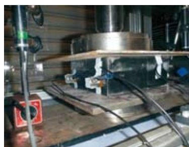
■ Acoustic Emission measurement which is one of the non-destructive testing of laminated rubber bearing.
