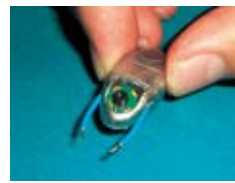
■ Capsule-Robot for diagnostic treatment with 30x15x8[mm] CCD camera and two forceps
