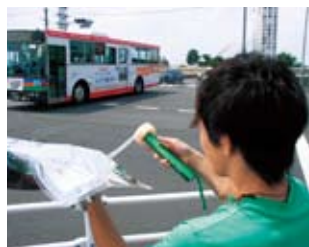
■ Air sample at a spot of roadside is collected. Pollution level of the target air is evaluated using both human noses and instruments.
