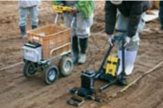
■ Quality assurance testing of soil compaction using a ground penetrating radar
