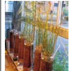
■ Landfill leachate treatment using lab-scale constructed wetlands
