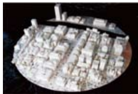
■ Researching reduction of heat island affect by reproducing a city in an experimental wind tunnel laboratory
