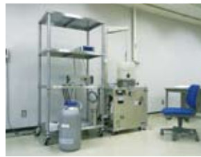
Thin organic film solar cells are created by evaporating organic molecular materials through being heated in the vacuum deposition equipment shown in the photo and then laminating it onto clear electrode substrates.
