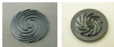
■ Silicon splitter impeller blade/reaction turbine blade of 10mm in diameter and fluid sealing structure (design point performance of rotation number of 90000rpm: pressure ratio 2, heat-insulating efficiency 0.5) that was experimentally produced by the processing technology with the micro machine system.
