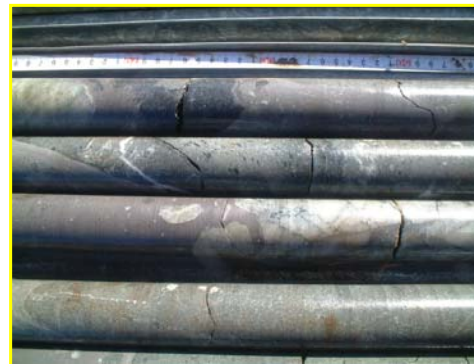
A typical example of the complicated lithology in the fault zone, with fragmented patches in every size, consisting of country rock (basaltic lava (hanging wall; light green) and quartzite (footwall; light gray)), fill-up with cataclasite (dark gray).
