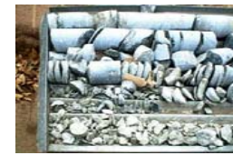
7m deep Photo 4. An example of drill core with borehole breakout
