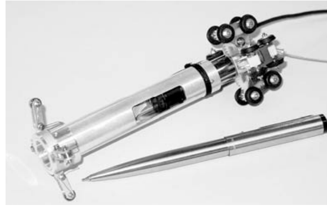
Fig. 4. Toshiba Corporation pipe robot
