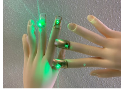
Fig. 15. Photograph of experimental setup of wireless power transfer scheme with dual-polarization-switching antenna and LED false nails.
