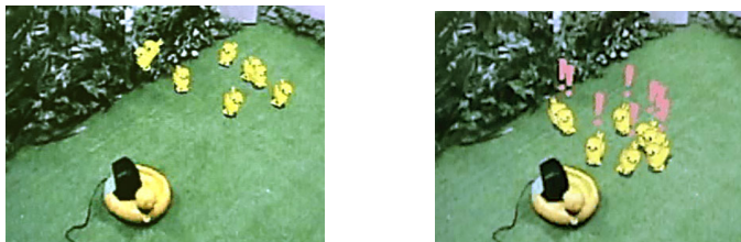
Fig. 17. Ducklings (CG) gather toward mother duck (real toy object with speaker) by using sound source localization in “Watch the Birdie!”
