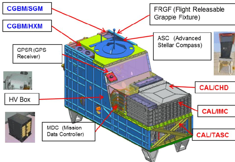
**FIGURE 1.** The CALET payload. On the ISS the payload will be installed in such a way to have open sky on top, Earth on bottom. The CALET Calorimeter (CAL) consists of Charge Detector (CHD), Imaging Calorimeter (IMC) and Total Absorption Calorimeter (TASC).
