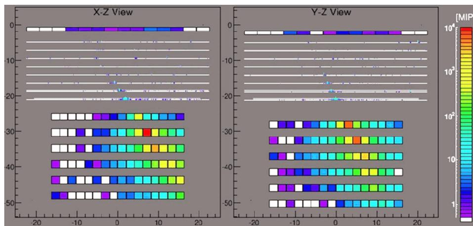
**FIGURE 4.** An example of an electron event display with an energy in the TeV region detected by CALET-CAL. One can see the top slate of CHD, 7 thin layers of IMC, followed by 6 thick layers of TASC. The left panel is the X-Z view and the right panel is the Y-Z view. The scale shown right is in the unit of MIP.
