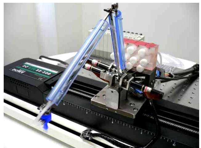
Fig. 10. Developed guide robot. Four DC servo rotational motors and one linear motor are built in the base part.
