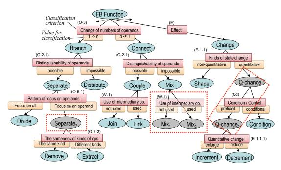
**Figure 4.** Reconciled Functional Basis (FB) with classification criteria defined in FOCUS/View (portion). This is logically modified according to these criteria. (the gray nodes have been inserted)
