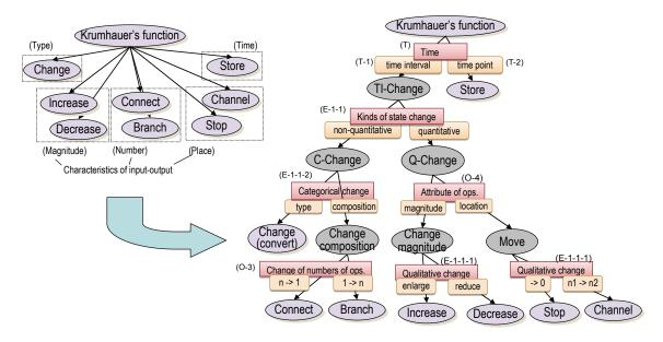
**Figure 6.** Classification criteria of Krumhauer's generally valid functions. (Left) Original classification [5], (Right) Re-organization using FOCUS/View with inserted terms (the gray nodes)
