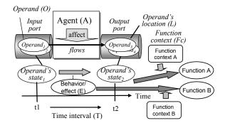
Figure 2. The base-model of function for FOCUS/View
