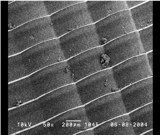
Fig.2 Fabricated cylinder lens using the mask shown in Fig.1
