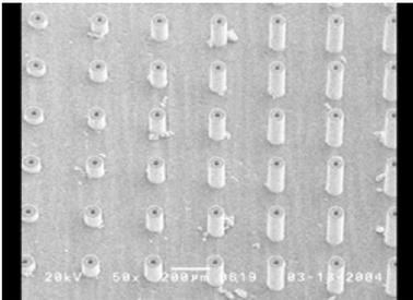
Fig. 4 Different aspect ratio structures obtained by the Gaussian intensity distribution of the x-ray source
