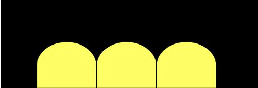
Fig.1 Semi-circle pattern LIGA mask for cylinder lens
