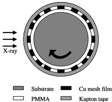
Fig.6 Rotation exposure principle
