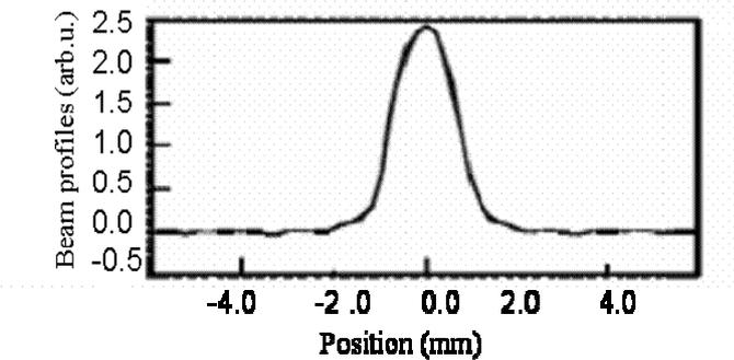
Fig. 3 X-ray Gaussian intensity distribution of x-ray source in Ritsumeikan University
