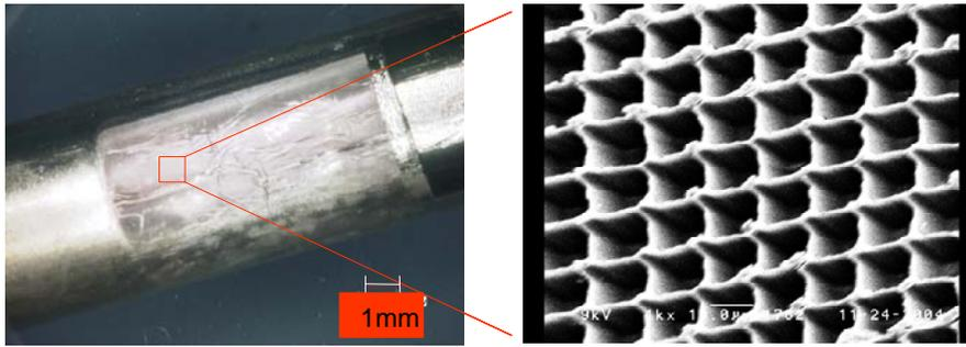
Fig.8 Photography of micro grating on cylinder surface
