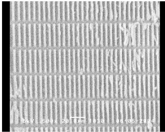
Fig.5 Micro gratings on a convex surface
