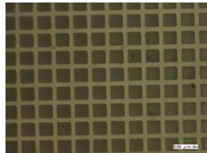
Fig.7 Copper mesh as LIGA mask
