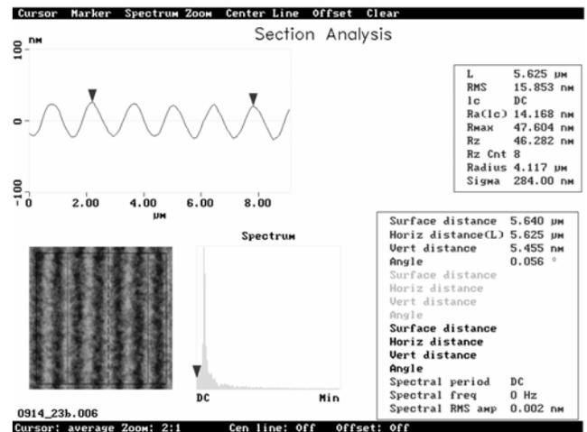
Fig.10 Cross sectional mapping measured by SPM at area (a) in Fig. 9. The height of the structure was 190 nm with dose energy in 0.184  $\text{kJ}/\text{cm}^3$ .
