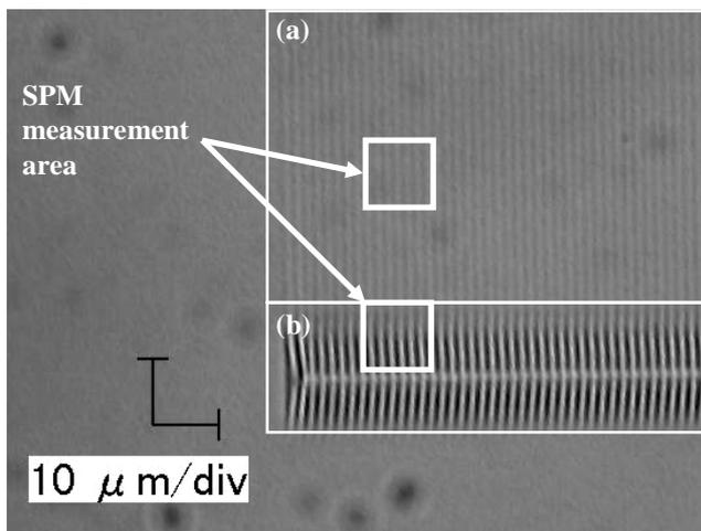
Fig.9 A top-view image of exposed structure, after developed at (a) turning position at the end of moving stage and (b) typical PCT exposed area.
