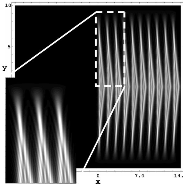
Fig.6 Top view of a simulated intensity distribution during a direct (static) exposure to the mask patterns
