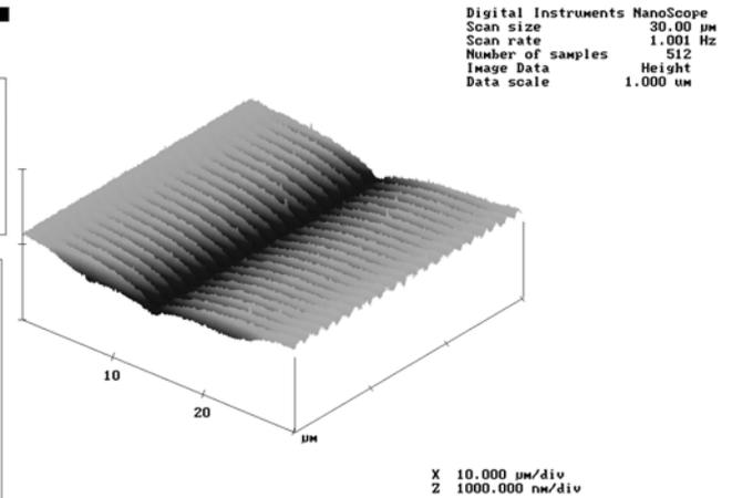
Fig.11 Cross section mapping measured by SPM Fig.12 3D view measured by SPM at (b) area. at (b) area.
