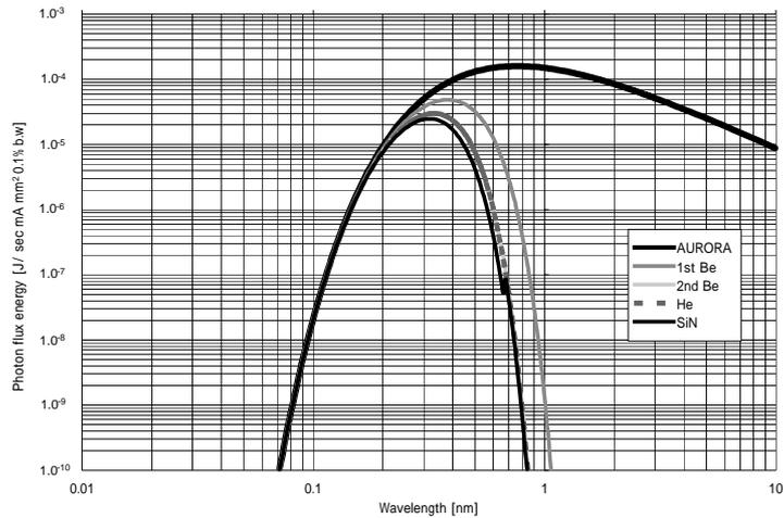
Fig.1 Spectrum of the SR beam line #13 of the AURORA
