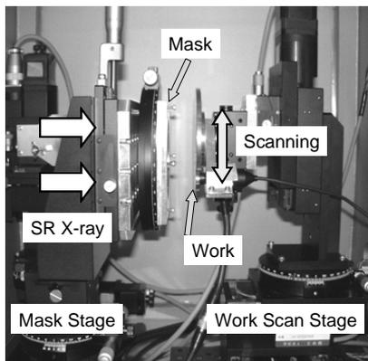
Fig. 2 The motorized stages in the exposure chamber for PCT process
