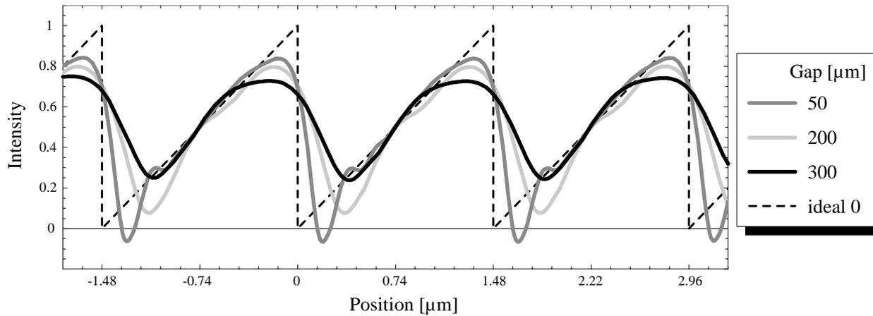
Fig.8 Calculation of X-ray intensity distribution in the resist from multi-wavelength. Data plotted from simulations for structure fabricated by the gaps; 50 $\mu\text{m}$ , 100 $\mu\text{m}$ , 200 $\mu\text{m}$ , 300 $\mu\text{m}$ . The broken line is the actual profile of replicated patterns.
