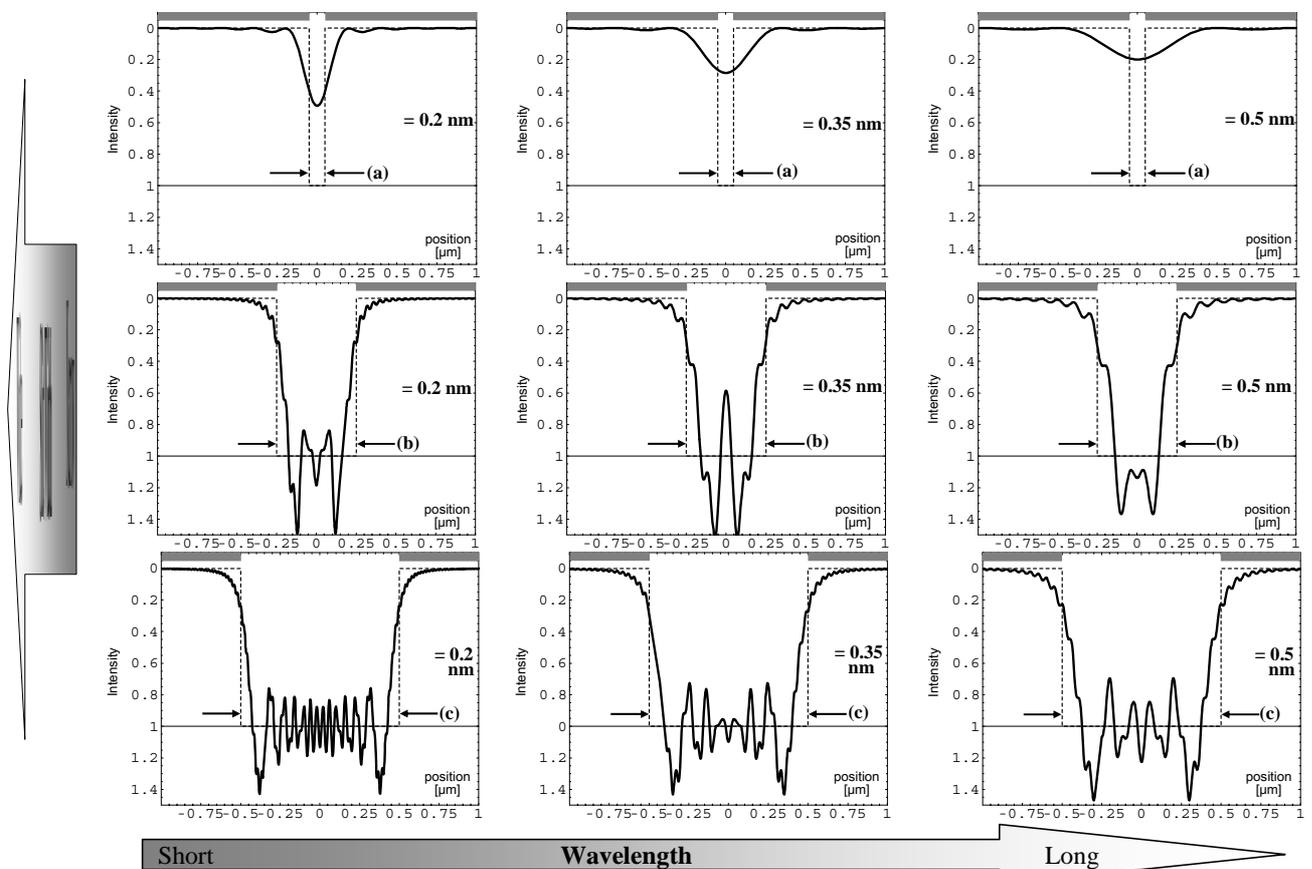
Fig.5 Simulated intensity distributions for three selected plane crossing a slit with the width of (a) 0.1  $\mu\text{m}$  (b) 0.5  $\mu\text{m}$  and (c) 1  $\mu\text{m}$ .
