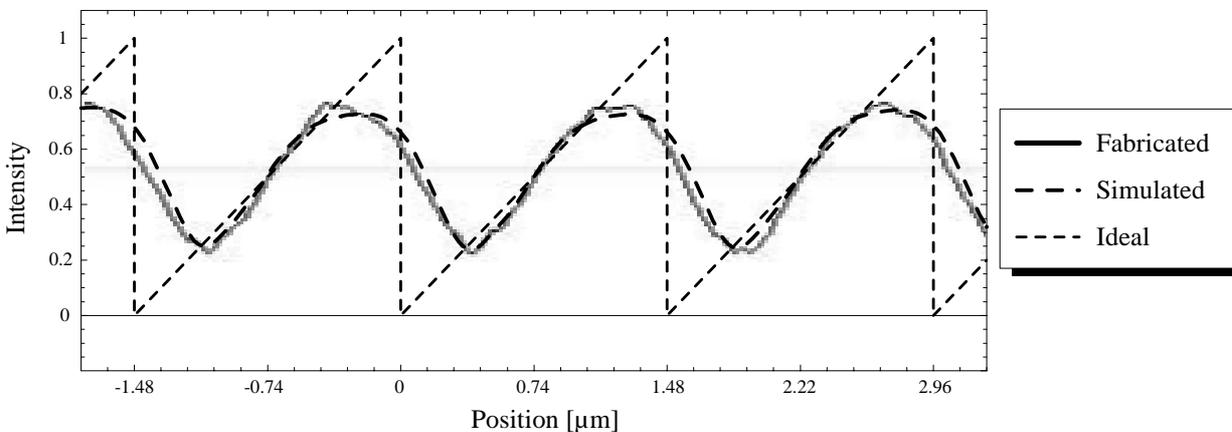
Fig.13 Calculation of the X-ray intensity distribution in the resist compared with the fabrication result.
