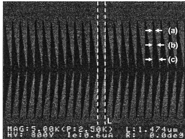
Fig.4 The triangular X-Ray mask-patterns.
