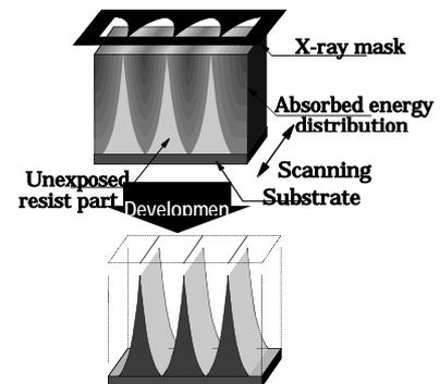
Fig. 3 The schematic of the PCT process.
