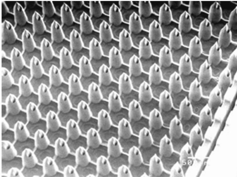
Fig. 1 Array of microneedles after optimizing hole-location and strength improvement
