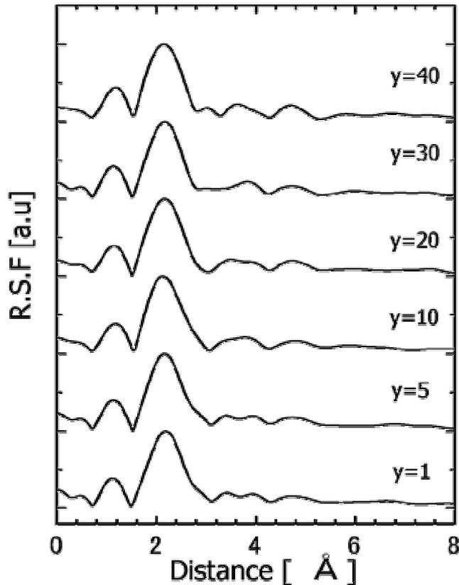
Figure 3 The radial structure functions obtained Ba L<sub>III</sub>-edge EXAFS spectra for Al<sub>2</sub>O<sub>3</sub>-99[50BaO-50B<sub>2</sub>O<sub>3</sub>] glasses.
