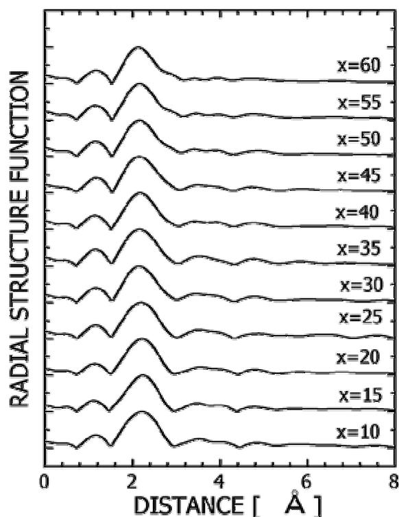
Figure 2 The radial structure functions obtained Ba  $L_{\text{III}}$ -edge EXAFS spectra for  $\text{Al}_2\text{O}_3-99[x\text{BaO}-(100-x)\text{B}_2\text{O}_3]$  glasses.
