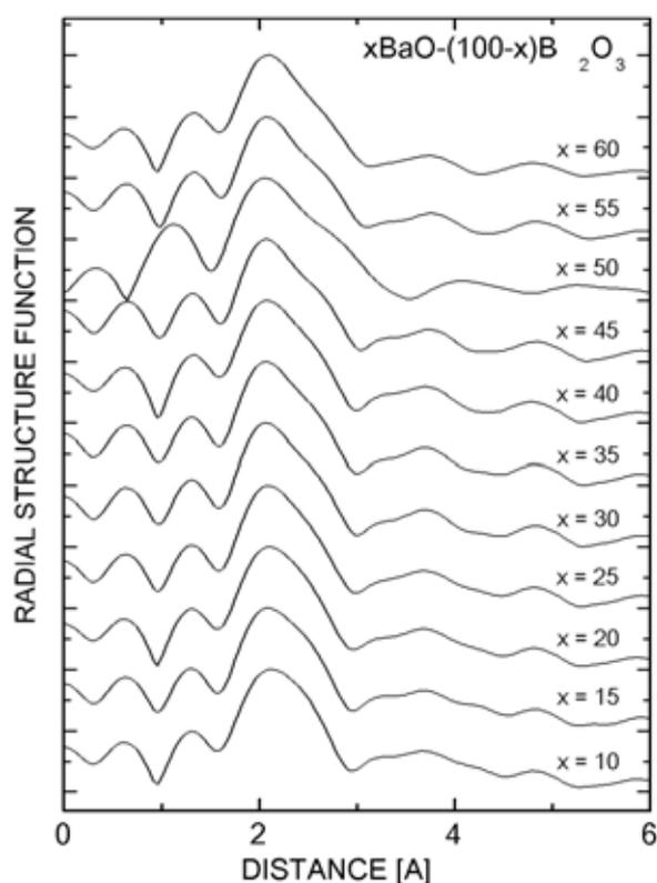
Figure 1 The radial structure functions obtained Ba  $L_{\text{III}}$ -edge EXAFS spectra for  $x\text{BaO}-(100-x)\text{B}_2\text{O}_3$  glasses.
