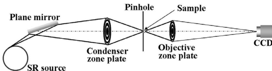
Fig.1 Schematic diagram of a RITS soft X-ray microscope
