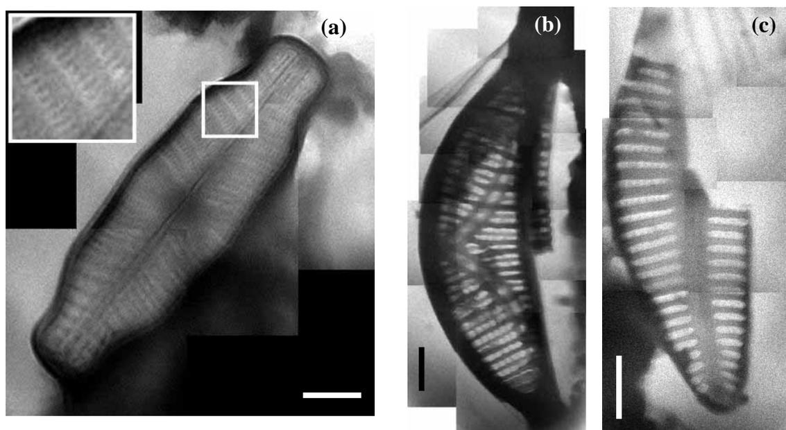
Fig.3 X-ray images of diatoms. (a)  $\lambda=2.4\text{nm}$ . Exposure was 10 minutes for each image. (b)(c)  $\lambda=1.9\text{nm}$ . Exposure was 30 seconds for each image. Bar= $2\mu\text{m}$ .
