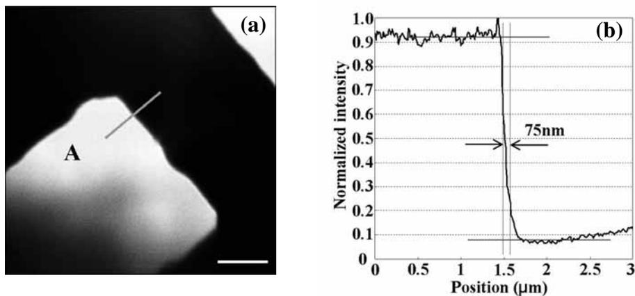
Fig.2 (a) X-ray image of a copper mesh (12.7 $\mu$ m/pitch). (b) Intensity profile of a line A. Bar=2 $\mu$ m.
