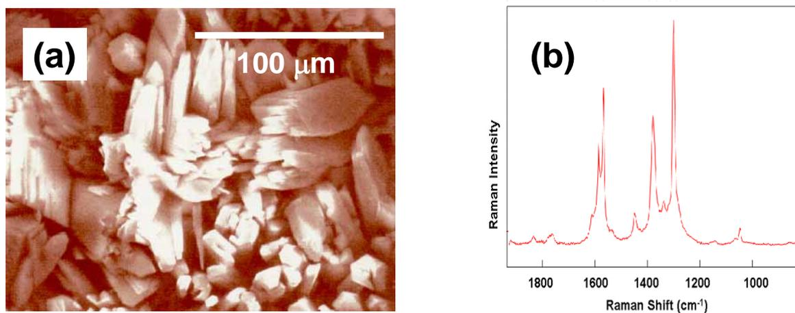
**Figure 2.** (a) SEM image of the micro crystals and (b) a Raman spectrum of these crystals.
