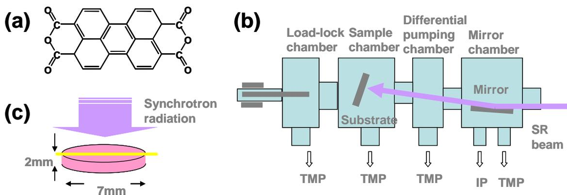
**Figure 1.** The molecular structure of PTCDA (a) and schematic representations of BL-14 (b) and synchrotron radiation to a pellet (c).
