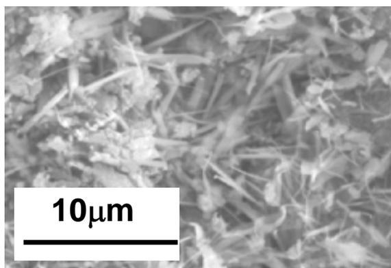
**Figure 3.** Needle crystals formed at the surface of a PTCDA/Na pellet after synchrotron radiation for 500 sec.
