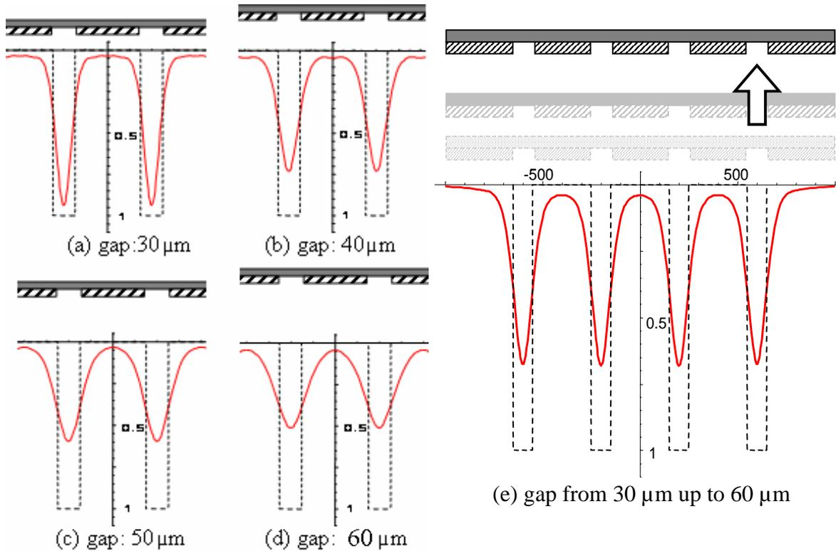
Fig. 7 The simulation results of x-ray intensity distribution
