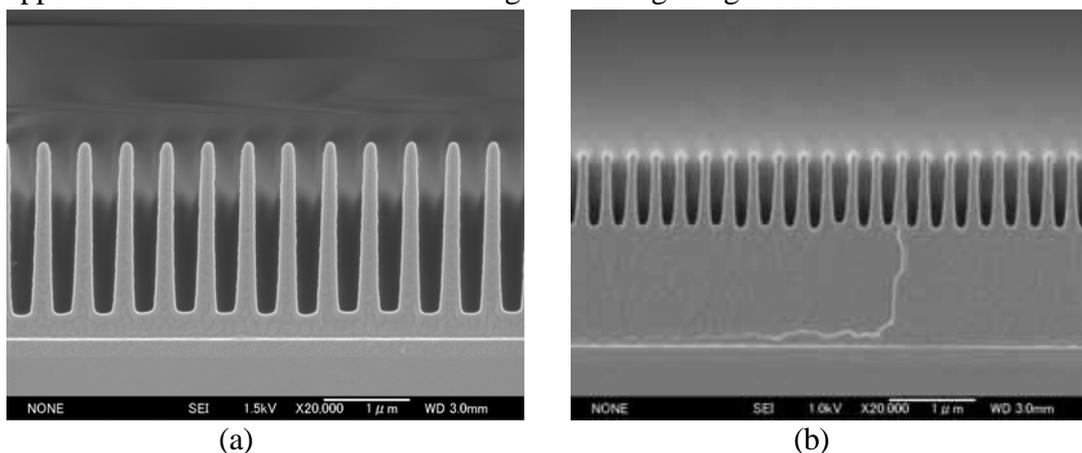
**Fig. 5** The grating with (a) 500 nm pitch and (b) 300 nm pitch
