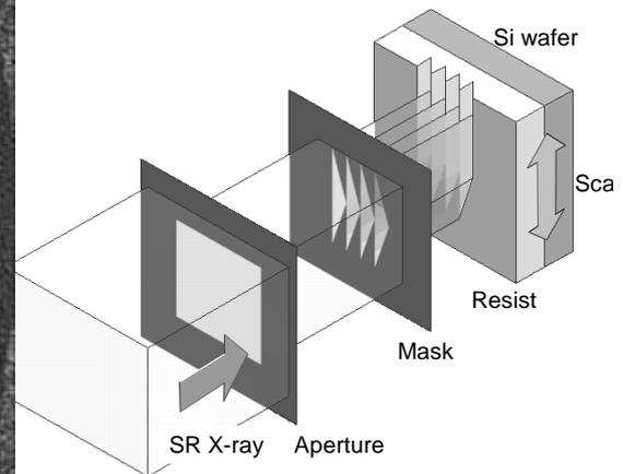
**Fig. 2** The schematic of the PCT exposing process
