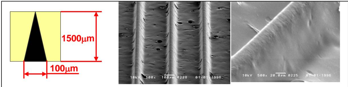
Fig.9 Mask pattern and SEM images of resulting structure from triangular mask (140°C)
