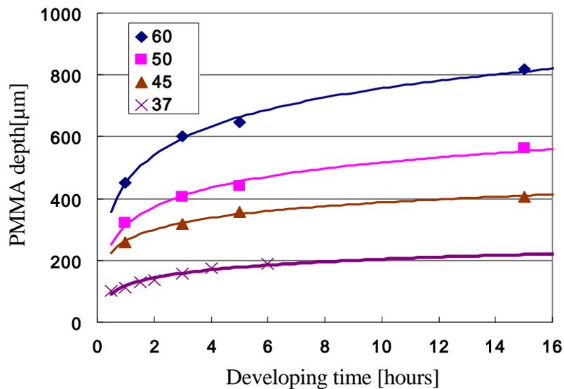
Fig. 5 Data plot of PMMA depth revealed by various developing temperatures against the time (the X-ray dose amount of 0.025 A.h)
