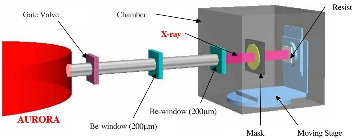
Fig. 1 The schematic of BL-15 and the stage system
