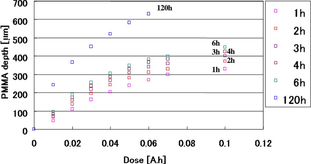
Fig. 2 General data plot used for PMMA exposed by SR from AURORA light source at BL-13 with developing temperature of 37°C.
