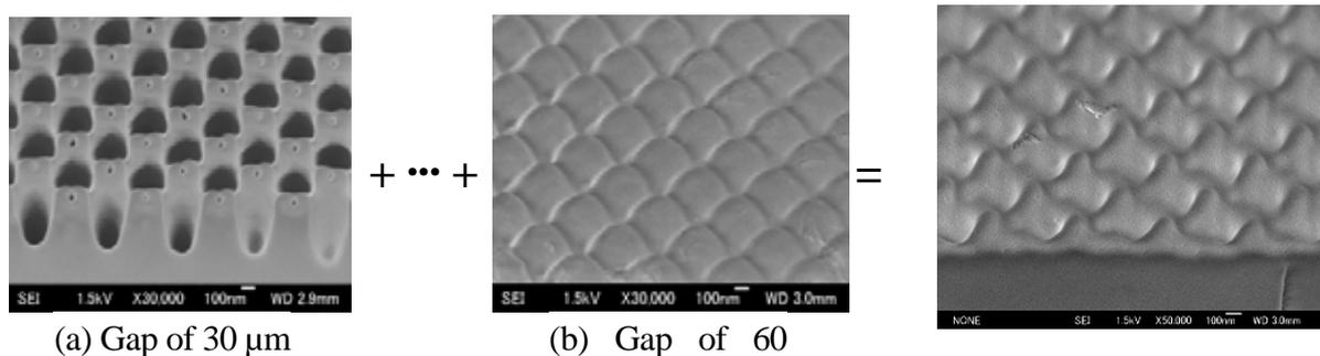
**Fig. 8** SEM photographs of 3D surface submicron array.
