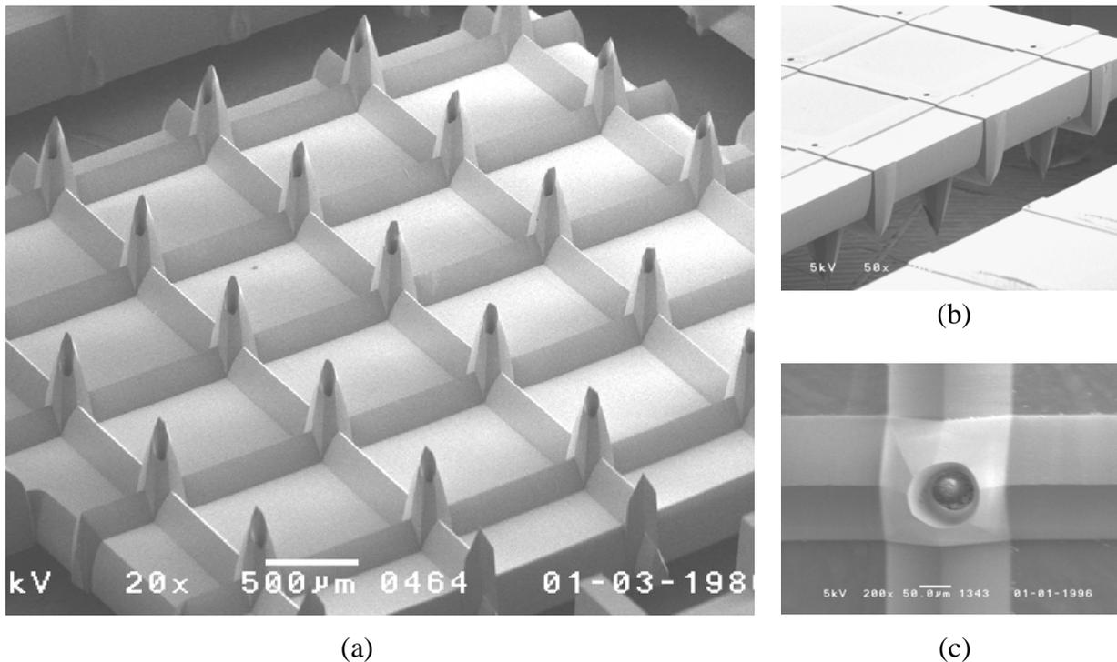
Fig. 1 Images of microneedle fabricated by PCT and Alignment exposures, (a) the microneedle array, (b) back side of the array and (c) incomplete hole observed.
