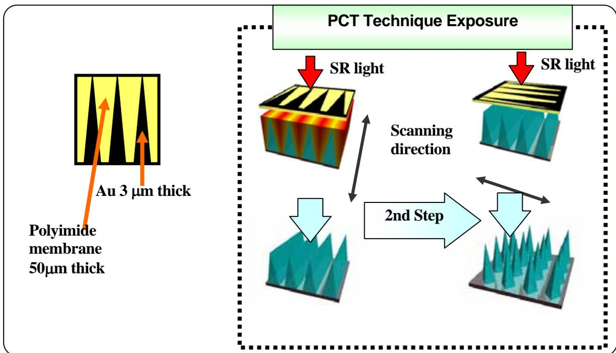
Fig.4 PCT technique exposure
