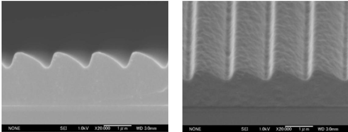
Fig. 6 The blazed grating with pitch of 1.5  $\mu\text{m}$
