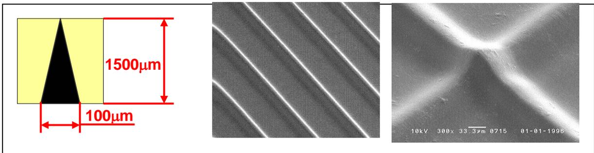
Fig.10 Mask pattern and SEM images of resulting structure from triangular mask (200°C)
