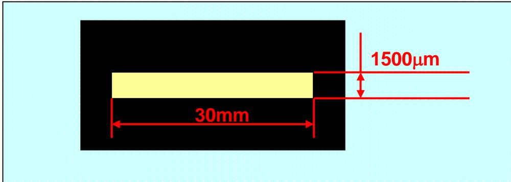
Fig.5 mask pattern and PTFE surface
