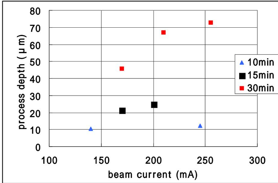
Fig.7 beam current VS the processing depth (200°C)
