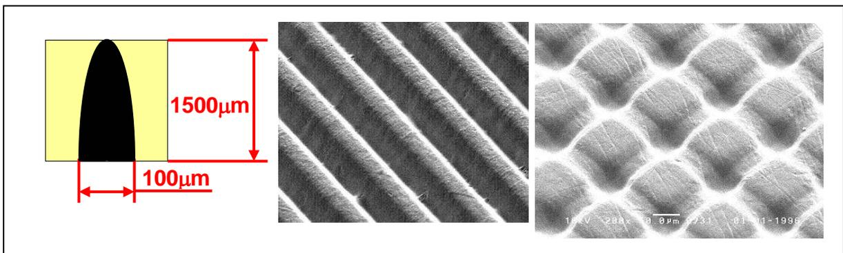
Fig.11 Mask pattern and SEM images of resulting structure from semicircular mask
