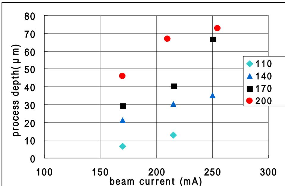
Fig.6 beam current VS the processing depth (30min)
