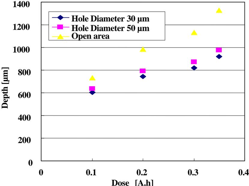
Fig. 9 Dose data for the hole-exposure for 10 hours development at 50 °C
