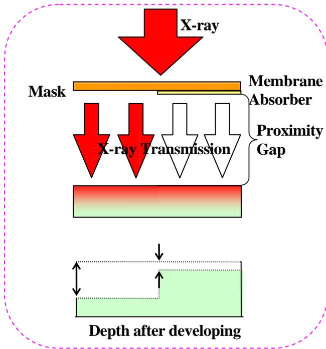
Fig. 3 Schematic of X-ray transmission through the mask
