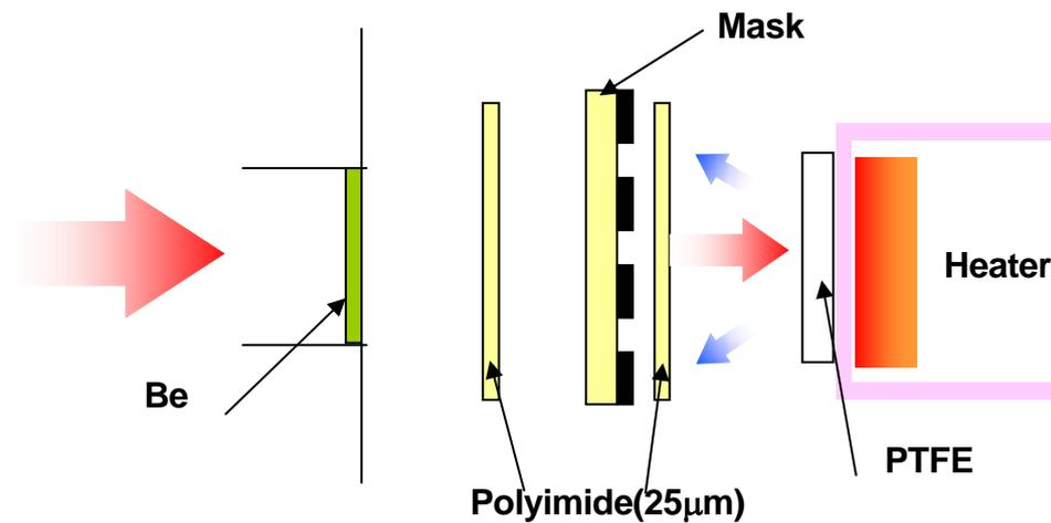
Fig. 3 The schematic of experimental system
