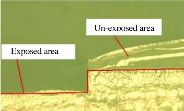
Fig. 7 Swollen surface of PMMA after developing by temperature at 55°C
