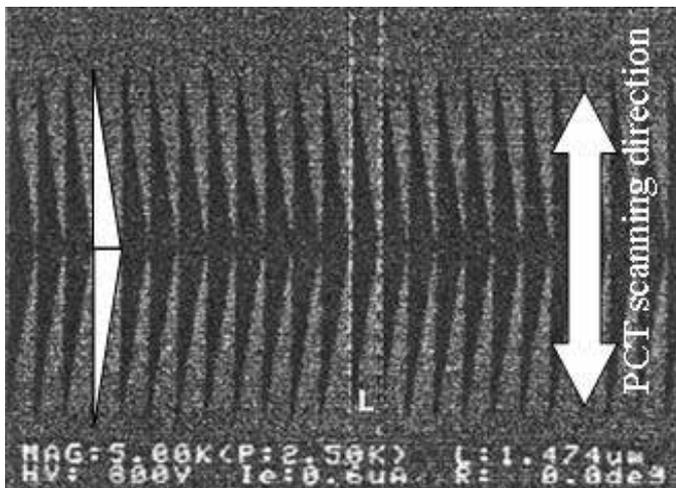
**Fig. 1** The SEM image of x-ray mask pattern for blazed grating
