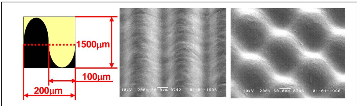
Fig.12 Mask pattern and SEM images of resulting structure from sine-curved mask
