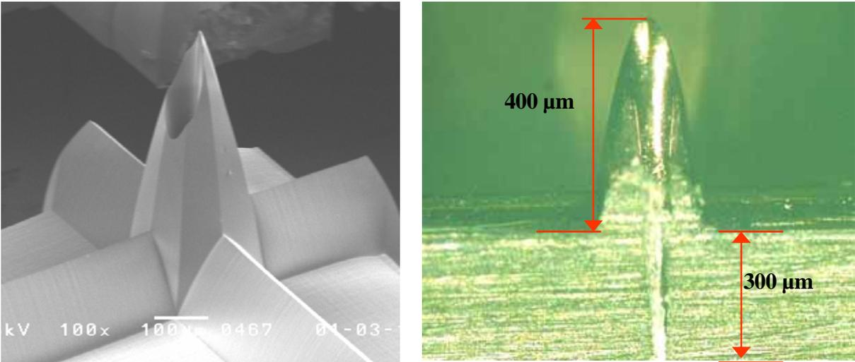
Fig. 10 Microneedle with desired configuration and completely through hole
