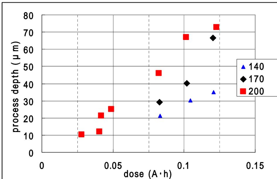
Fig.8 dosage VS processing depth
