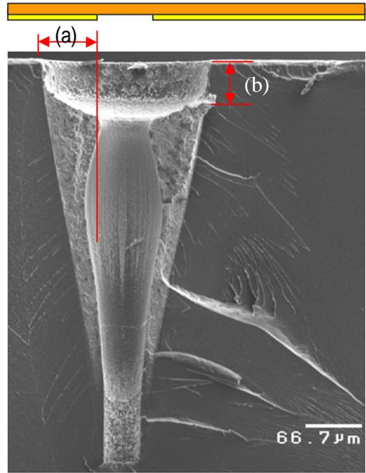
Fig. 4 Effects of (a) proximity gap and (b) X-ray transmission through absorber
