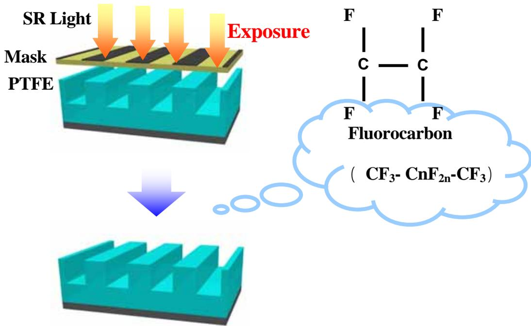
Fig. 2 PTFE etching mechanism
