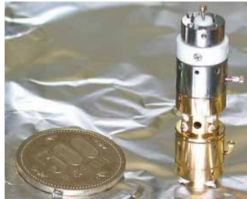
Fig. 2. Close-up of the electron gun designed for scanning electron microscopy.
