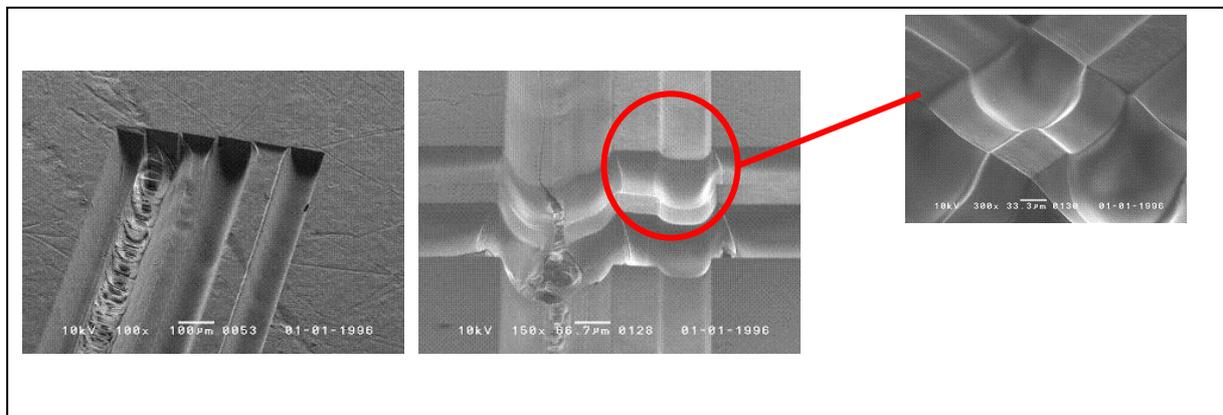
Fig.3 SEM images of PTFE structures
