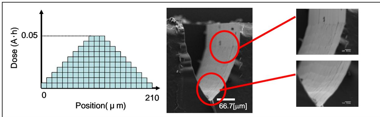
Fig.2 energy distribution and fabricated structure
