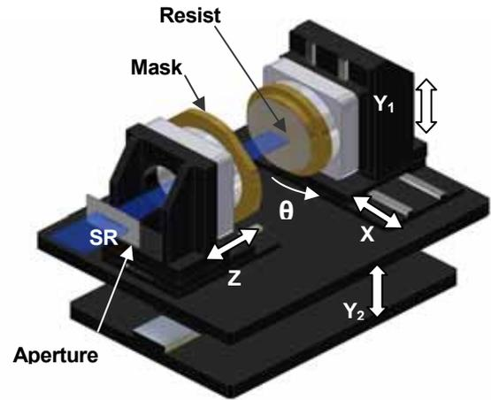
Fig.1 Multi-functional exposure stage at BL-5
