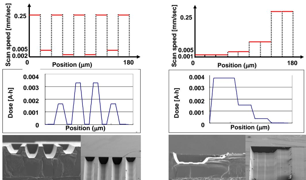
Fig.7 Scan speed, energy distribution, structures
