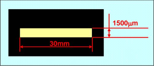
Fig.2 Mask pattern 1500µm x 30mm
