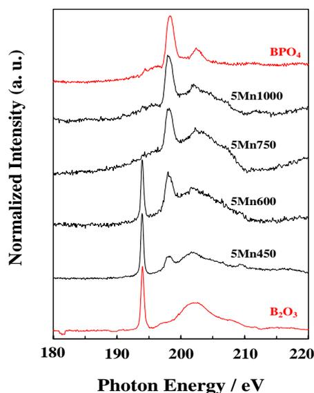
Figure 1. B *K*-edge XANES spectra of  $\text{Mn}^{2+}$ -doped  $\text{BPO}_4$  and reference samples. Sample of  $5\text{MnO}\cdot 95\text{BPO}_4$  heat treated at 450 °C is, for example, indicated as 5Mn450 °C.
