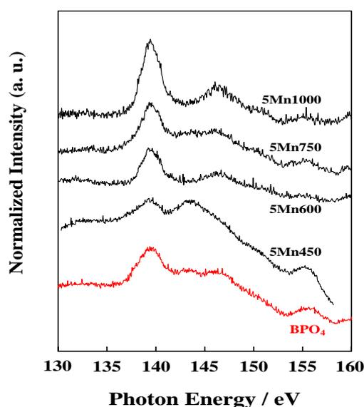
Figure 2. P *L*-edge XANES spectra of  $\text{Mn}^{2+}$ -doped  $\text{BPO}_4$  and a reference sample of  $\text{BPO}_4$ . Sample of  $5\text{MnO}\cdot 95\text{BPO}_4$  heat treated at 450 °C is, for example, indicated as 5Mn450 °C.
