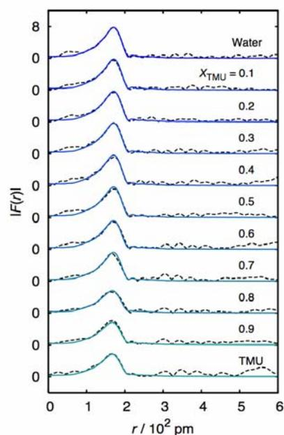
**Fig. 6** The radial structure functions  $|F(r)|$  for Mn(II) ion in water-TMU solvents, phase shift uncorrected. The dashed lines are experimentally obtained ones, and the solid lines are calculated ones.
