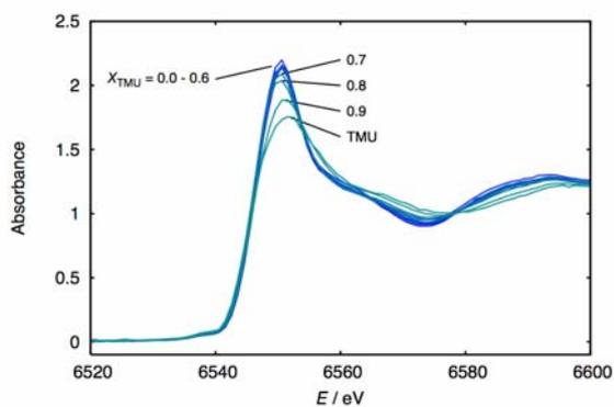
**Fig. 3** The normalized XANES spectra of Mn(II) ion in water-TMU solvents.
