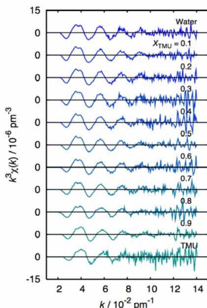
**Fig. 5** The extracted EXAFS oscillations in the form of  $k^3\chi(k)$  for Mn(II) ion in water-TMU solvents.
