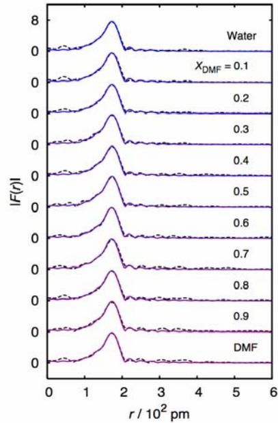
**Fig. 2** The radial structure functions  $|F(r)|$  for Mn(II) ion in water-DMF solvents, phase shift uncorrected. The dashed lines are obtained experimentally, and the solid lines are calculated.
