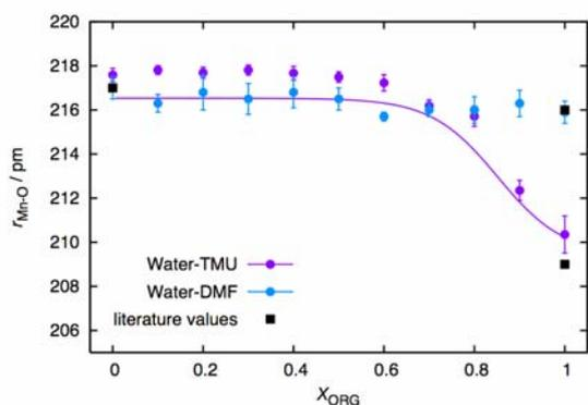
**Fig. 7** The Mn-O distances obtained by EXAFS analysis. Filled squares show the values from refs. 1 and 2.
