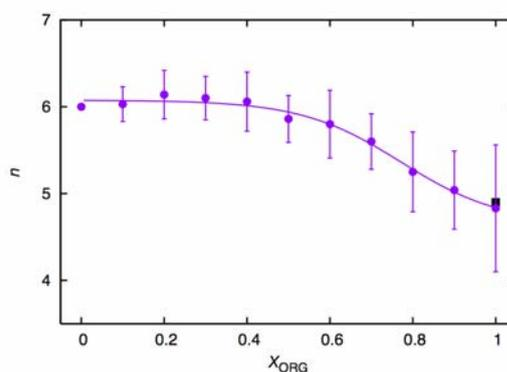
**Fig. 8** The coordination number of Mn(II) in the water-TMU solutions. Filled square shows the value from ref. 2.
