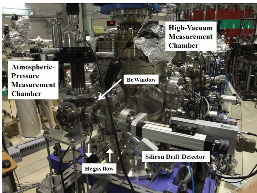
**Fig. 2.** Photograph of the atmospheric-pressure measurement chamber.
