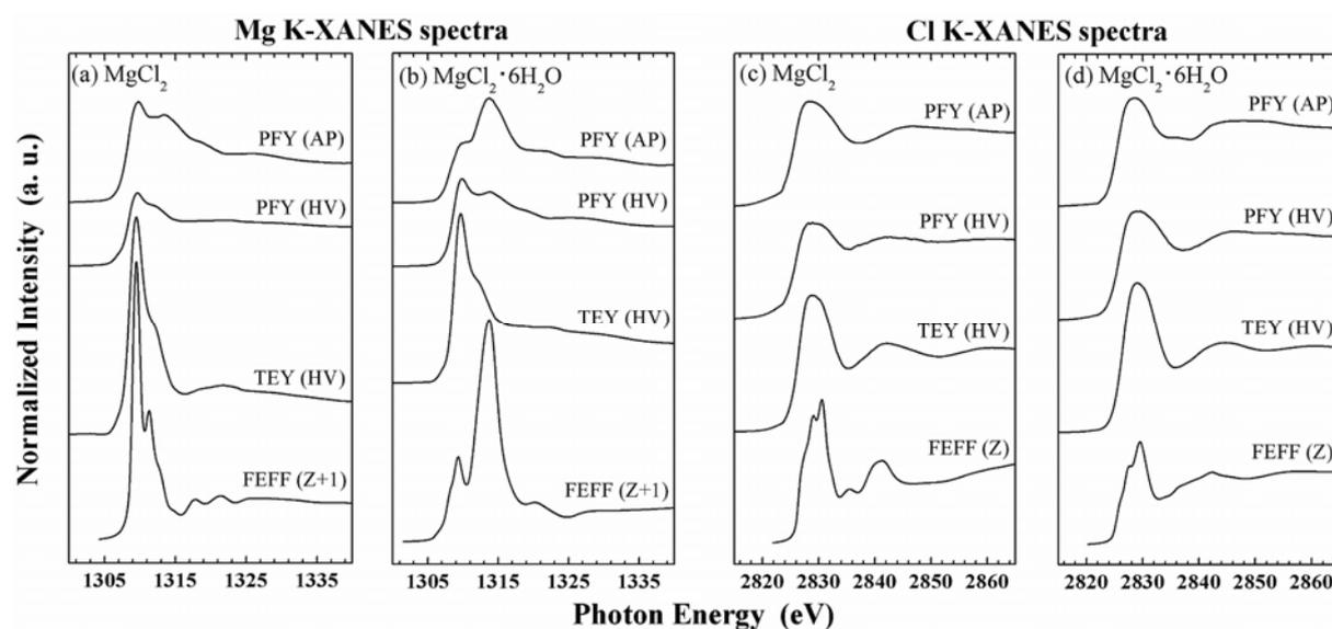
Fig.4. Observed and simulated Mg and Cl K-XANES spectra. (a) Mg K-XANES spectra of MgCl<sub>2</sub>, (b) Mg K-XANES spectra of MgCl<sub>2</sub>·6H<sub>2</sub>O, (c) Cl K-XANES spectra of MgCl<sub>2</sub>, (d) Cl K-XANES spectra of MgCl<sub>2</sub>·6H<sub>2</sub>O. Simulated XANES spectra by FEFF of (a) and (b) used the Z+1 approach to obtain a better agreement with the observed spectra [7].
