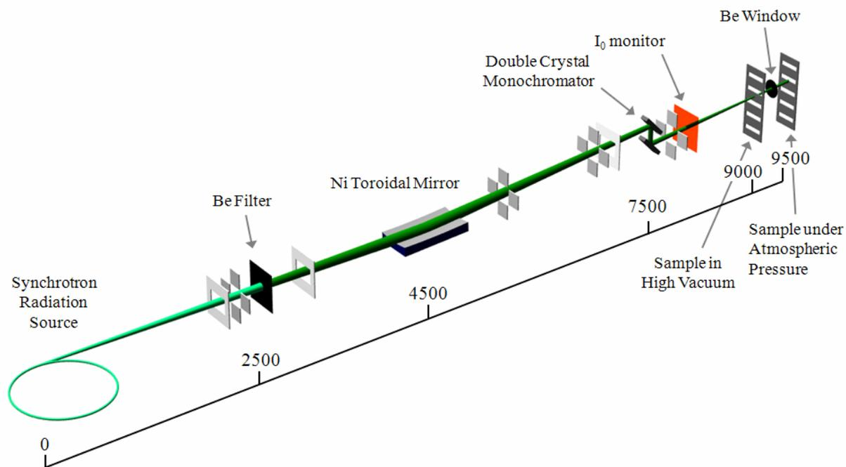
**Fig.1.** The schematic configuration of the BL-10.
