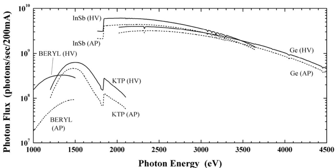
**Fig.3.** Observed photon fluxes on the sample position in HV (solid line) and under AP (dashed line).
