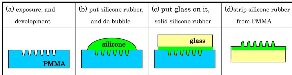
**Fig.8** The PMMA mold process using silicone rubber
