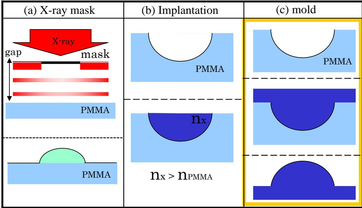
**Fig.6** The examined methods to make the micro lens
