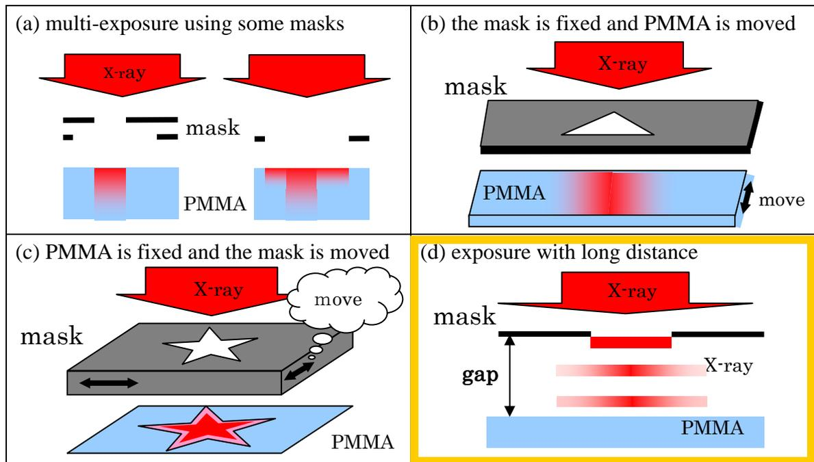
**Fig.1** Several methods to fabricate a 3D structure
