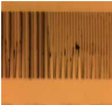
Fig.6 Microscope photo: Collapse of the structure (Line width 20\mu\text{m} , Space width 20\mu\text{m} ) after development.
