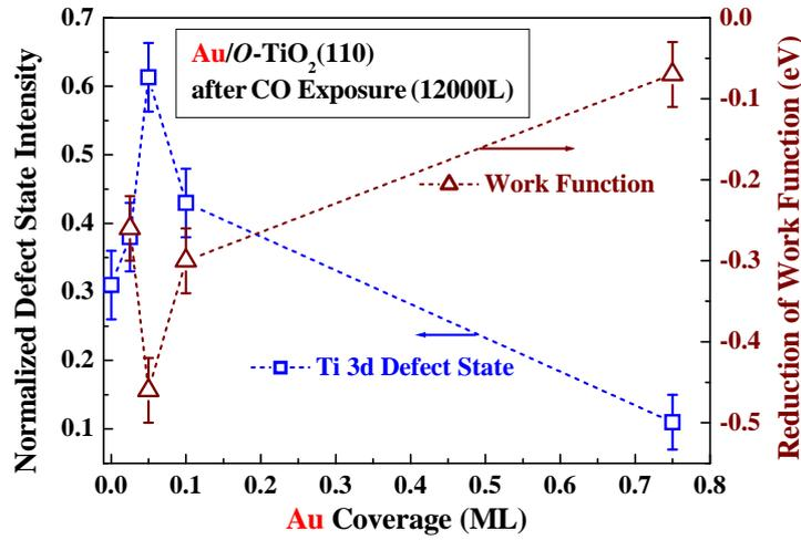
Fig. 8. Defect state intensity (open squares) normalized by that for *R*-TiO<sub>2</sub>(110) indicated for Au/*O*-TiO<sub>2</sub>(110) after CO exposure of 12000 L as a function of Au coverage. Right side axis: Reduction of work function (open triangles) relative to that for Au(111) indicated for Au/*O*-TiO<sub>2</sub>(110) after CO exposure of 12000 L as a function of Au coverage.
