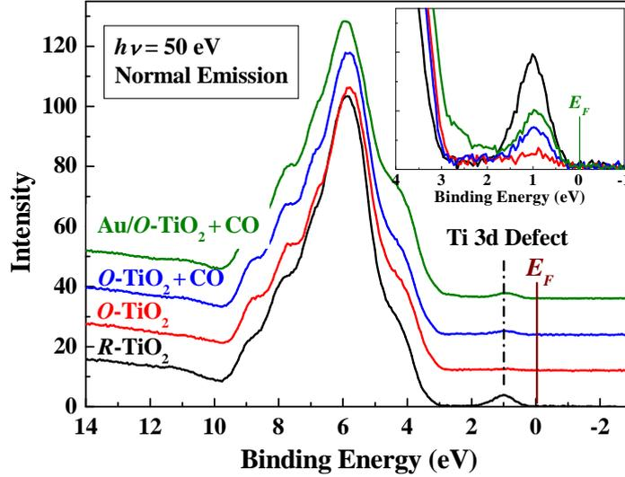
Fig. 3. UPS spectra observed at photon energy of 50 eV under normal emission condition for  $R\text{-TiO}_2(110)$ ,  $O\text{-TiO}_2(110)$ , and  $O\text{-TiO}_2(110)$  and  $\text{Au}(0.05 \text{ ML})/O\text{-TiO}_2(110)$  after CO exposure of 12000 L. Binding energy ( $E_B$ ) is scaled from Fermi level ( $E_F$ ). Inset indicates magnified spectra of Ti 3d defect state.
