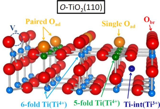
Fig. 1. Ball and stick model for  $O\text{-TiO}_2(110)$ . Orange balls represent  $\text{O}_{\text{ad}}$  atoms and  $V_{\text{O}}$  is bridging O vacancy. Small dark-blue ball denote Ti interstitial acting as an n-type donor.
