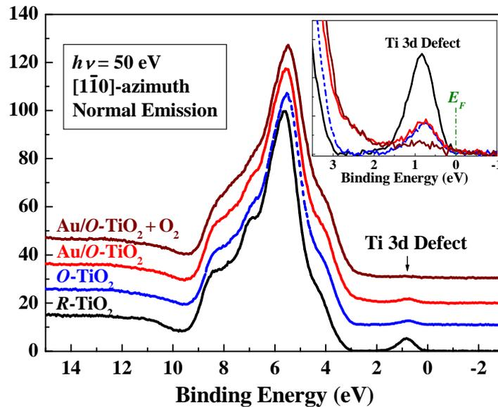
Fig. 6. UPS spectra observed for  $R$ -,  $\text{O-TiO}_2$ ,  $\text{Au}(0.08 \text{ ML})/\text{O-TiO}_2$ , and  $\text{Au}(0.08 \text{ ML})/\text{O-TiO}_2$  after  $^{18}\text{O}_2$  exposure of 1000 L at RT. Inset indicates magnified spectra around Ti 3d defect state. Sheet resistance of  $\text{TiO}_2$  support employed here is  $\sim 100 \Omega/\square$ .
