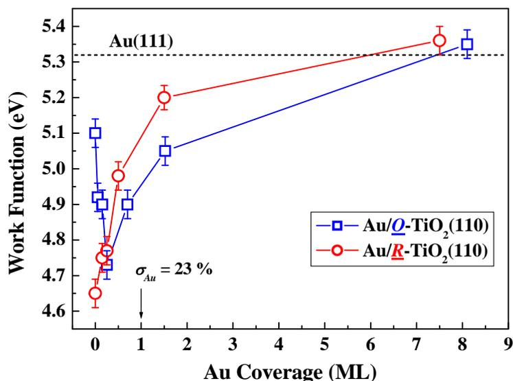
Fig. 7. Work function measured for Au/O-TiO<sub>2</sub>(110) (open squares) and Au/R-TiO<sub>2</sub>(110) (open circles) as a function of Au coverage. Dashed line indicates the work function of Au(111) (5.31 eV)[38]. Error bars originate from experimental uncertainty of  $\pm 0.04$  eV.
