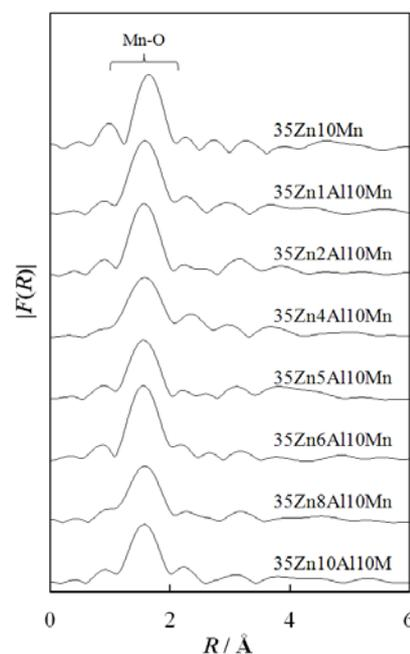
Fig. 4. Radial structure functions,  $|F(R)|$ s, of 35ZnxAl10Mn glasses.
