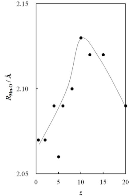
Fig. 8. MnO addition dependence on  $R_{Mn-O}$  in 35ZnzMn glasses.
