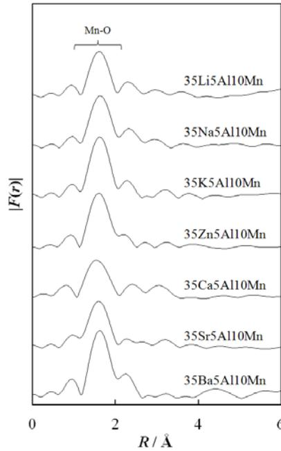
Fig. 2. Radial structure functions,  $|F(R)|$ s, of 35M5Al10Mn and 35M'5Al10Mn glasses.
