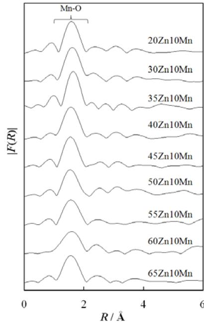
Fig. 5. Radial structure functions,  $|F(R)|$ s, of  $y\text{Zn}10\text{Mn}$  glasses.
