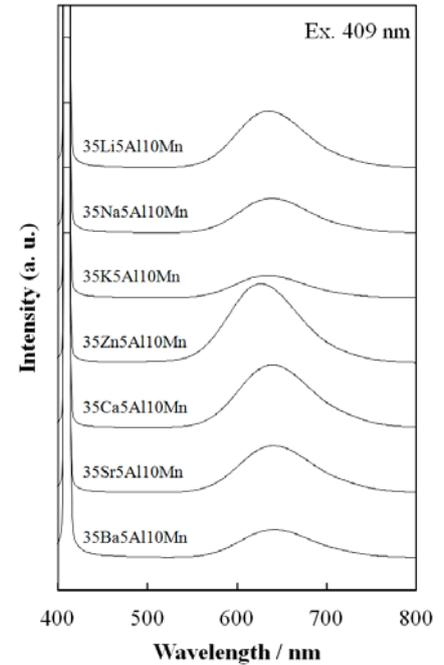
Fig. 3. Fluorescence spectra of 35M5Al10Mn and 35M'5Al10Mn glasses under excitation of 409 nm.
