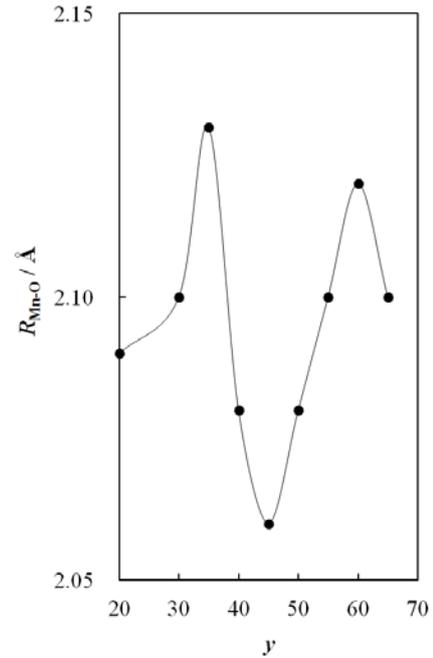
Fig. 6. Glass composition dependence on  $R_{\text{Mn-O}}$  in  $y\text{Zn}10\text{Mn}$  glasses.
