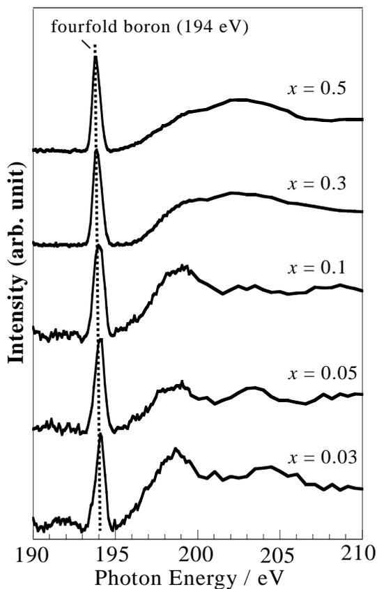
Fig.1. B K-edge XANES spectra of  $\text{Li}_2\text{MnSi}_{1-x}\text{B}_x\text{O}_4$ .
