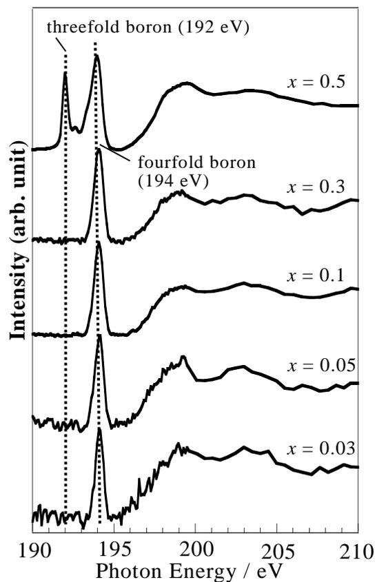
Fig.2. B K-edge XANES spectra of  $\text{B}_x\text{-Li}_2\text{MnSiO}_4$ .
