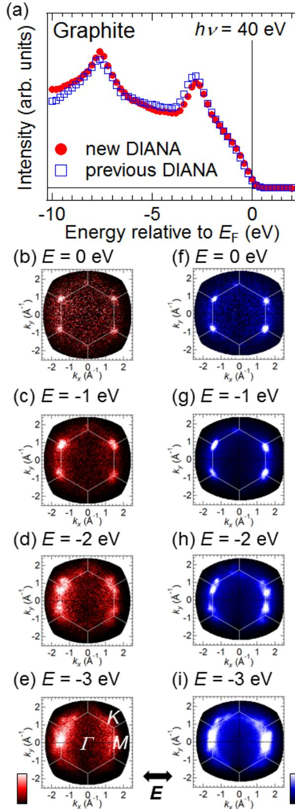
**Fig. 2** 2D-PES results of graphite. (a) Angle-integrated spectra. (b-e) 2D-PIADs obtained by the new DIANA. (f-i) 2D-PIADs obtained by the previous DIANA.
