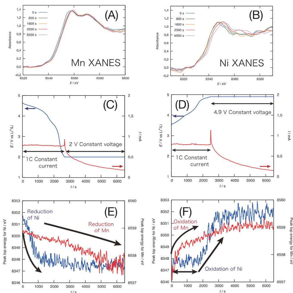
**Fig. 5** XANES spectra of charging process for Mn (A) and Ni K-edge (B); Electric current and cell voltage for the discharging process (C) and the following charging process (D); Time-course of the energy of the white line peak for the discharging process (E) and the charging process (F).
