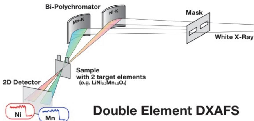
Fig. 1 Conceptual image of double-element DXAFS instrument.
