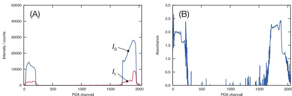
**Fig. 4** The raw data of the transmitted X-ray intensities measured by the DE-DXAFS instrument for the  $\text{LiNi}_{0.5}\text{Mn}_{1.5}\text{O}_4$  cathode sheet (A) and the X-ray absorbance at the Mn and Ni K-edges calculated by taking  $\ln(I_0 / I_t)$  (B).
