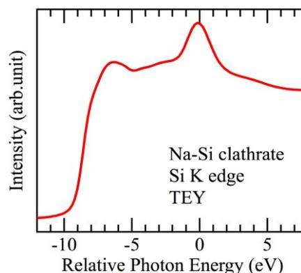
**Fig. 2** XANES at Si K edge in TEY mode. The origin of the relative photon energy was taken at the main peak of Si K XANES of  $\text{SiO}_2$ , the photon energy of which is around 1845 eV. The 0-eV peak presumably comes from the epoxy adhesive around the sample.
