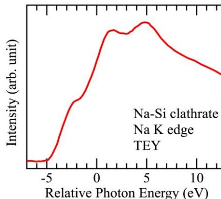
**Fig. 1** XANES at Na K edge in TEY mode. The origin of the relative photon energy was taken at the main peak of Na K XANES of NaCl, the photon energy of which is around 1075 eV.
