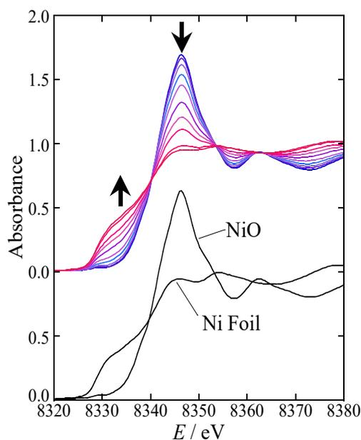
**Fig. 1** XANES change during the pretreatment process from room temperature to 700 °C under H<sub>2</sub> atmosphere.
