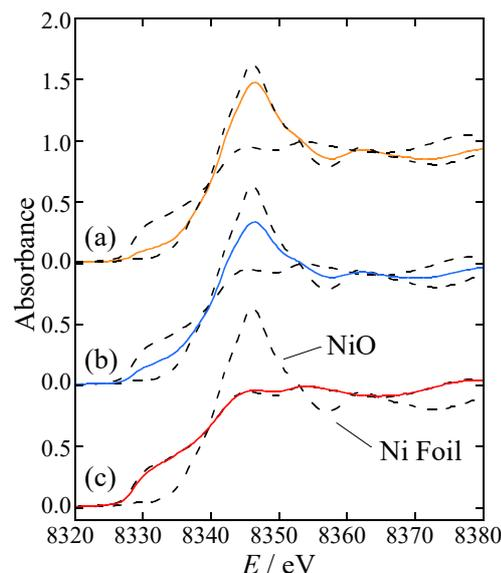
**Fig. 2** XANES spectra of SiO<sub>2</sub>-supported Ni catalysts with various composition. The quenched temperature during the reduction process was 300 °C (a), 336 °C (b), and 700 °C (c). The reference XANES spectra of Ni foil and NiO are given for comparison (dashed lines).
