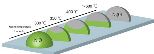
**Fig. 5** The reduction mechanism of the NiO particle supported on SiO<sub>2</sub>.
