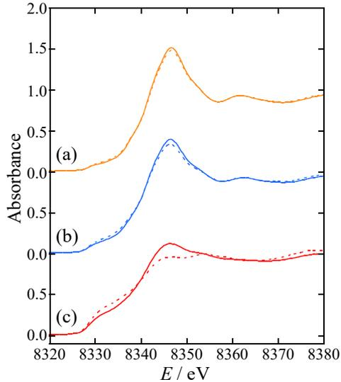
**Fig. 3** XANES spectral change of the Ni particle with different proportion of metallic Ni(0) by the O<sub>2</sub> exposure at room temperature. The reduction composition was 19% (a), 41% (b), and 100% (c). The dash and solid lines represent the XANES spectrum before and after the O<sub>2</sub> exposure, respectively.
