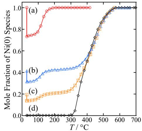
**Fig. 4** The mole fraction change of the Ni(0) species as a function of temperature during the TPR process after the O<sub>2</sub> exposure at room temperature. The reduction composition was 100% (a), 41% (b), 19% (c), and no reduction (d).
