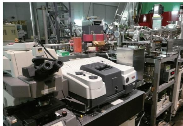
**Fig. 37.** Infrared Spectro-microscopy beamline (BL-15). Center: FT-IR (Nicolet 6700) and left: Microscopy (Continuum XL).
