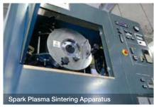
Sinters non-equilibrium powders through rapid heating, allowing sintering of materials such as ceramics and metals making use of their non-equilibrium conditions.
