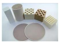
Various test specimens of porous solid electrolytes.
