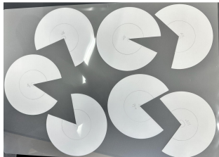
Fig.1 Kent paper with center corner cut out.
