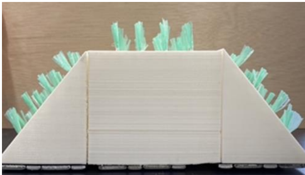
Fig.3 New type artificial reef with water plants models attached
