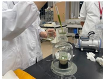
Fig.4 Suction filtration with Celite performed before titration to dilute the color
