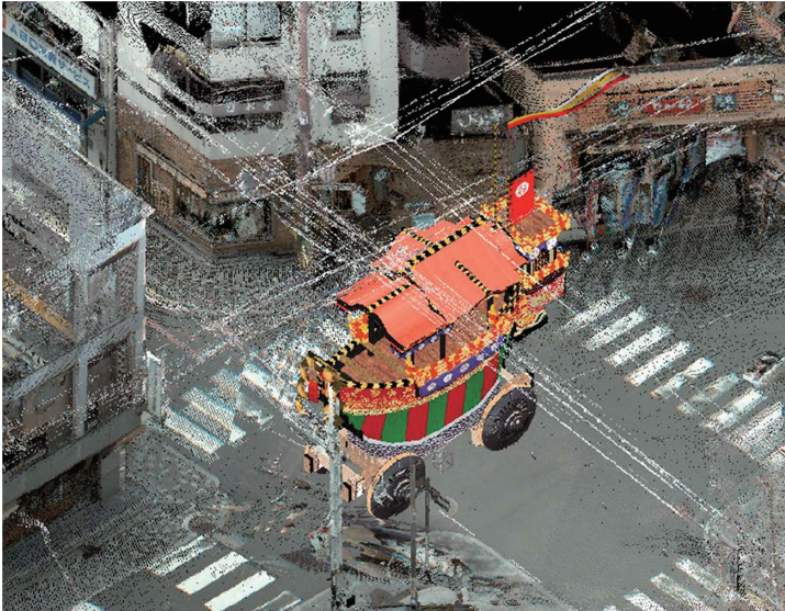
Figure 7. Point cloud of the Ofune-hoko float ( 9.7 \times 10^6 points) placed in the scene of Sanjo Street. Source: Author
