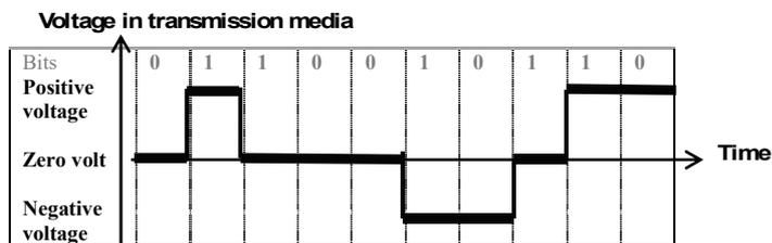
The example to illustrate changes of voltage for MLT-3 (Multi-Level Transmit).
