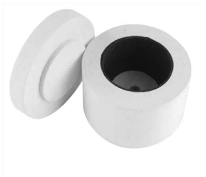
Figure 2. Camera image of the Microwave Kiln used for the low-temperature (250 °C) alkali fusion reaction
