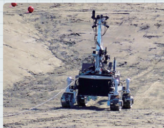
Lunar surface simulation field site (Nippon Yakin Kogyo Co., Ltd.) The rover was developed as part of the Ministry of Land, Infrastructure, Transport and Tourism's "Space Construction Innovation Project."
