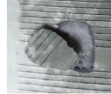
Fig.5 After freezing 10 times, part of the surface of the tiles chipped off.
