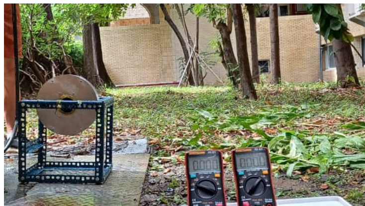
Figure 1: The overall experimental setup of the micro-hydroelectric generator, including digital multimeters for data recording in an outdoor environment (In KSHS)
