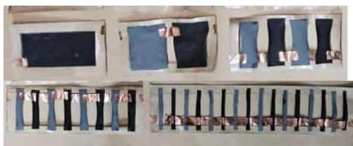
Image 4: Batteries with different segmentation
