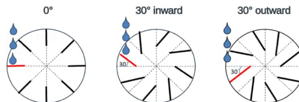
Figure 4: Comparison of blade setting angle
