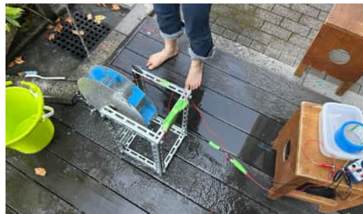
Figure 3: The overall experimental setup of the waterwheel-type generator, including a generator and voltmeter connected to it in an outdoor environment (In WUHSHS)
