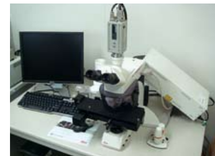
The laser microdissection apparatus: magic tweezers able to isolate a variety of cell groups
