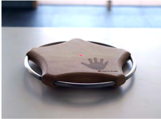
Figure 8: Tetsuaki Baba's Freqtric Drums project. The device creates music signals based on the human body's electrical conductivity.
