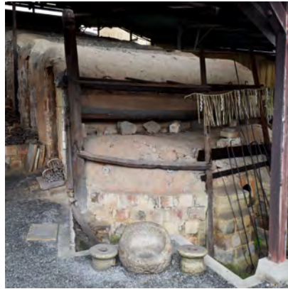
Figure 5: The kiln at the back of Kawai's house in Kyoto, built in the Noborigama style.
