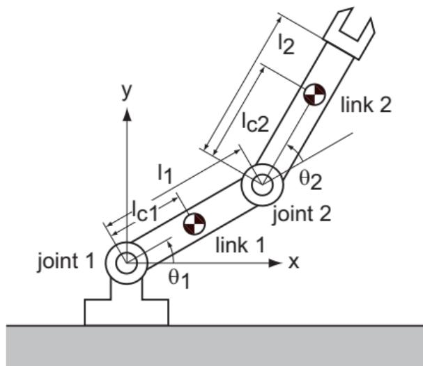
two link open link mechanism
