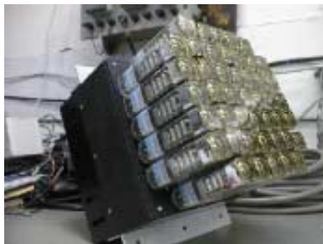
図 5 Photomultipliers of the camera system.
