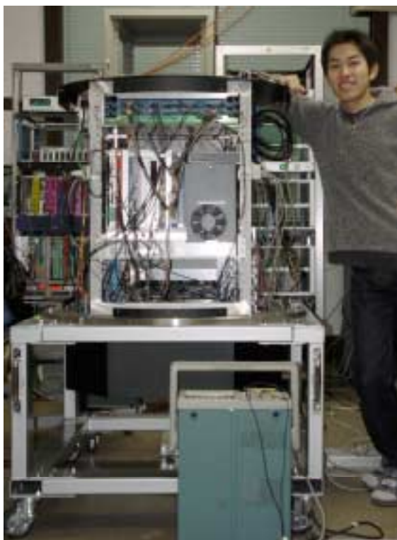
図 4 The gamma-ray camera in its final form (without a cover).
