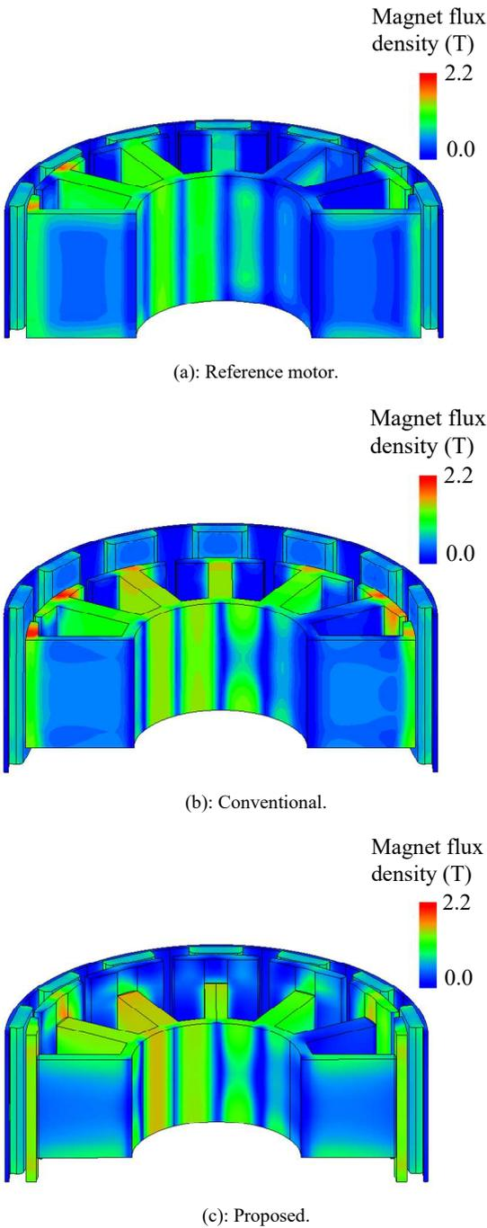
Fig. 6. Magnetic flux density on no-load condition.
